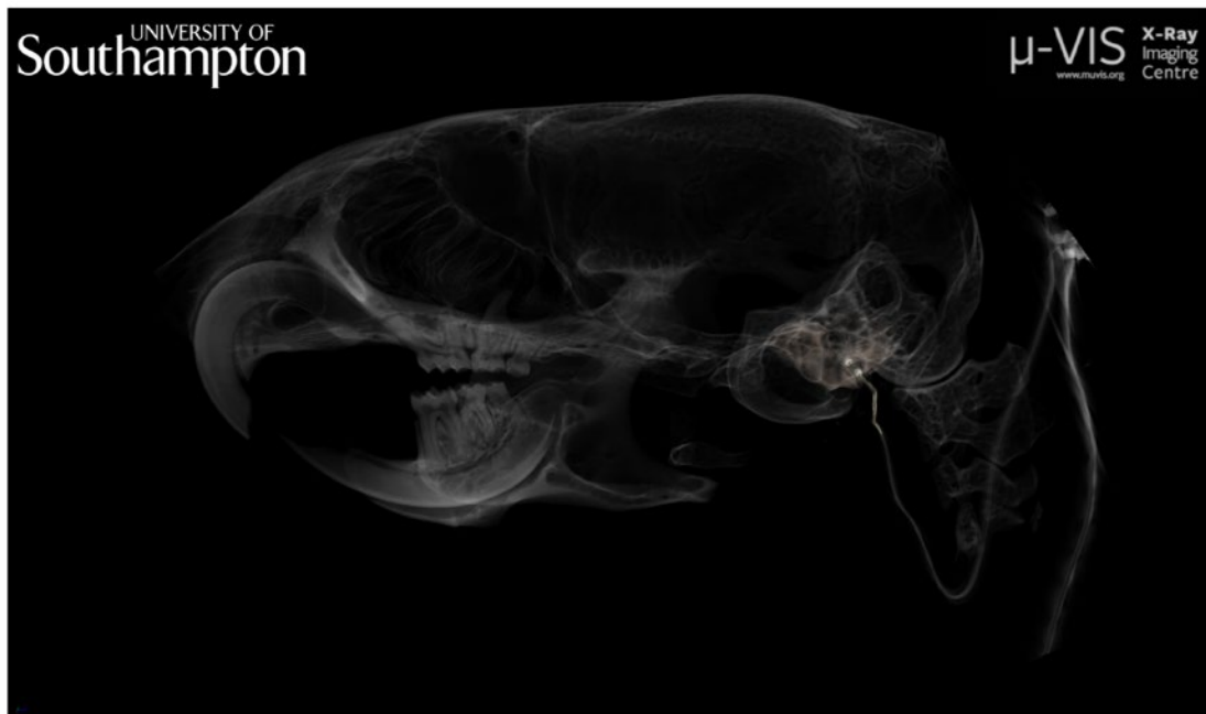
Figure 5.11 Whole mouse skull with electrode array implanted into the cochlea from a 12 \mu m resolution scan of TN516 visualised using VG Studio Max software
