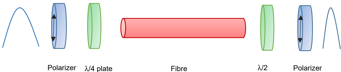
Fig.3.2.4 The basic structure of the NPR.
