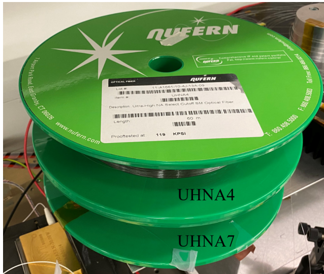
Fig. 4.2.4 Photo of the normal dispersion fibre coils. Top: Nufern UHNA4, Bottom: UHNA7.
