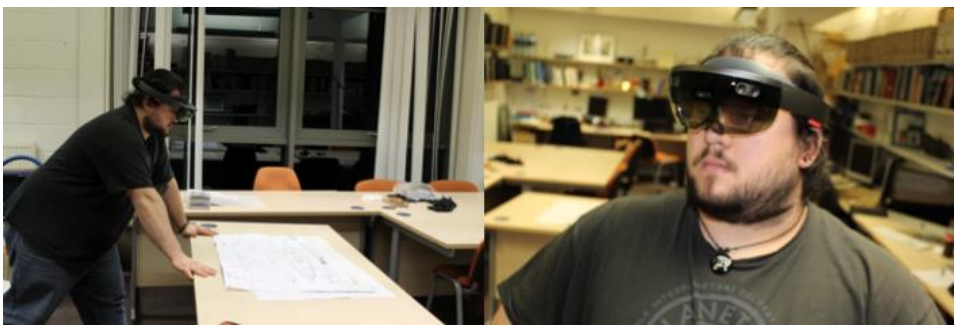
Figure 4.6 Head mounted display, HoloLens, used throughout the case study. Image courtesy of author.
