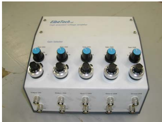
Fig. 12: External preamplifier with five independent channels and programmable gains.
