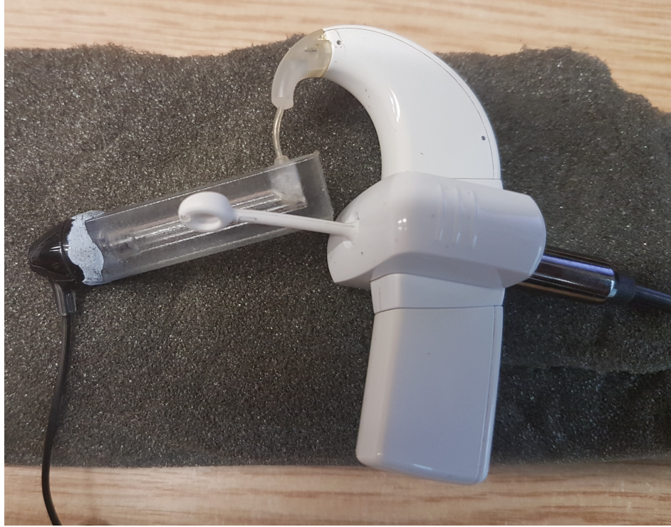
Figure 3.1: Picture showing a cochlear implant connected to a Listening Check and the custom enclosure
