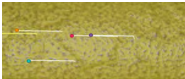
Figure 11: A simulation showing the tracking of features to achieve visual odometry.
