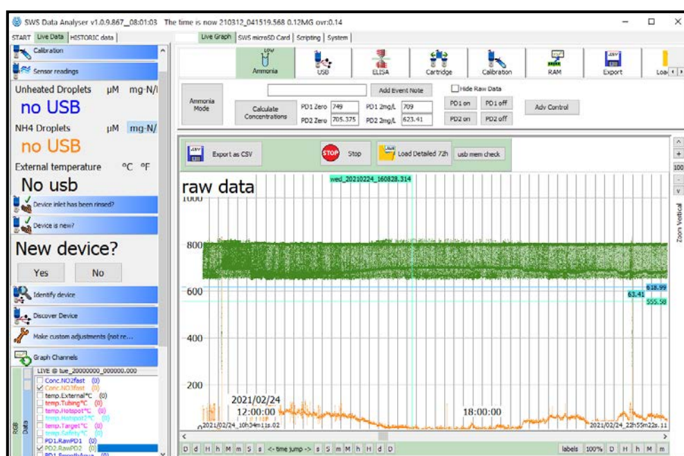
Figure 125. Screenshot of GUI displaying raw light intensity data (in green) and a concentration profile of ammonium (orange).
