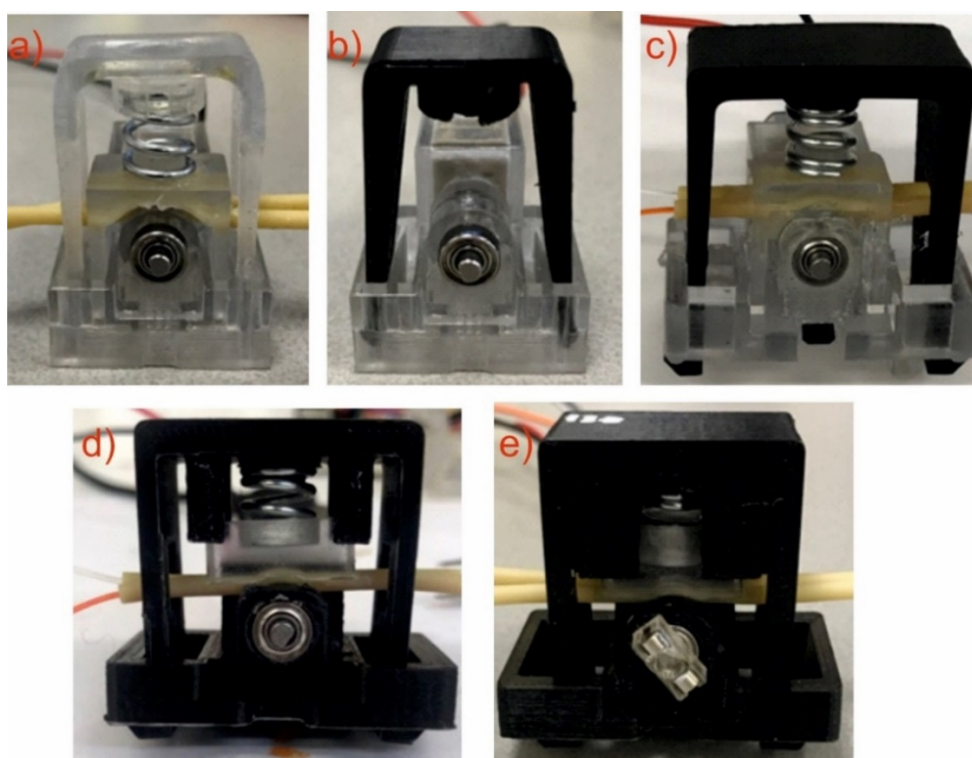
Figure 127. Photographs of 3D printed assemblies of the single spring pump showing the evolution to the current working version. (a) Entire pump printed using 'VeroClear' material in glossy finish. (b) Replaced top cap in (a) using more flexible black PLA printed one. (c) Expanded the design to make it sturdier. (d) Modular pumped and top cap modified to adjust to the new pump bed design. (e) Final design with more restricted top cap to allow only vertical motion of the pump bed and also modified chassis for easier insertion of top.
