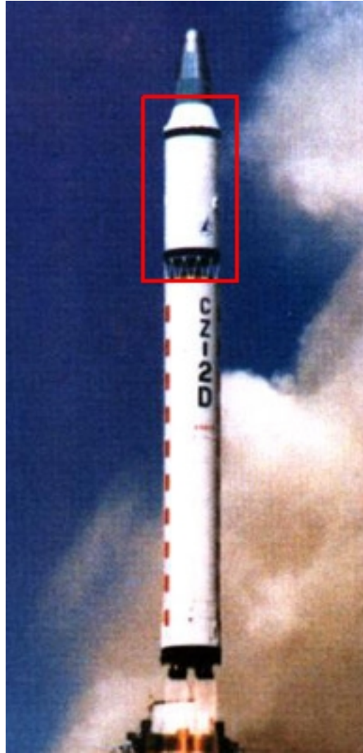
FIGURE 7.2: A CZ-2D launch vehicle with the upper stage that remains on-orbit indicated by a red box.
