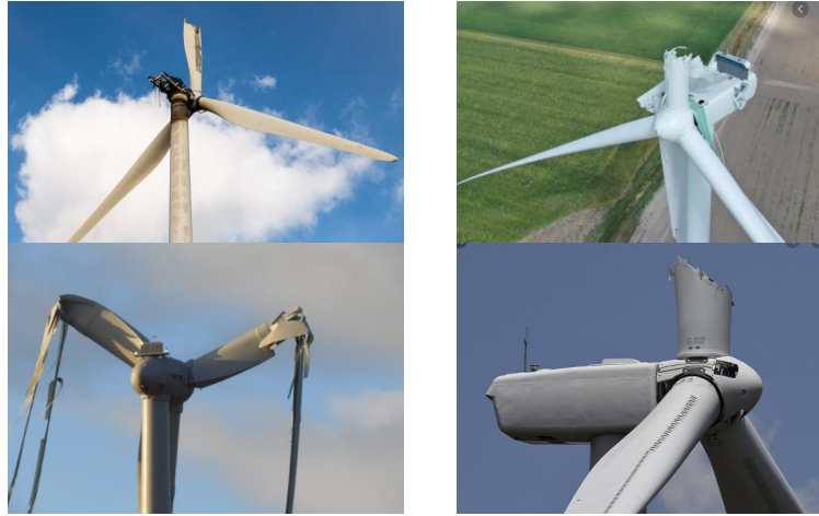
Figure A.1: Failed Wind turbine blades at the root and transition region obtain from google pictures, www.weatherguardwind.com/wind-turbine-blade-dielectric-protection/ date access 25th November 2020.
