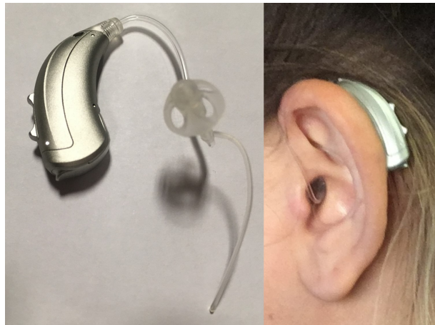
FIGURE 3.5: Photographs of the Signia Contrast S+ device used.
