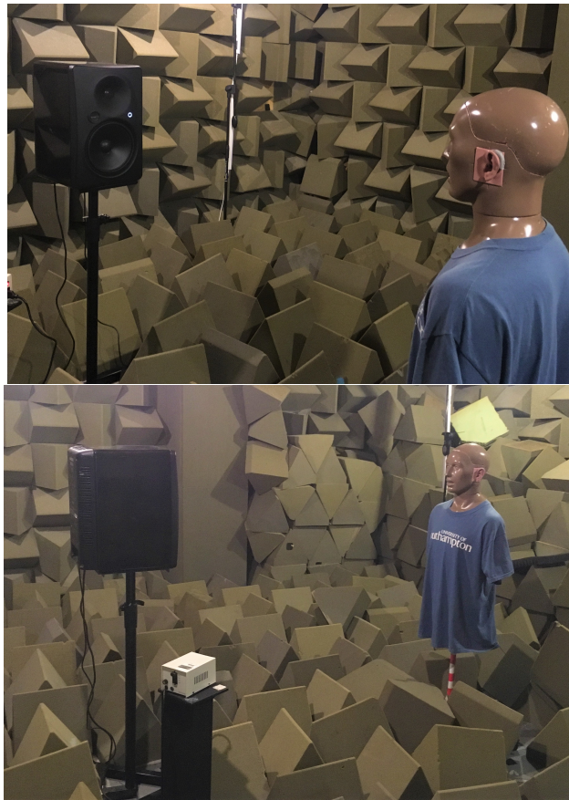
FIGURE 3.2: Photographs of the recording set-up with KEMAR.
