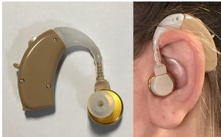
FIGURE 3.7: Photographs of the FoKe FK-162 amplifying device used.
