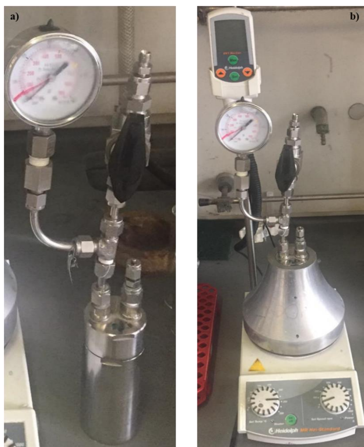
Figure 2-17. Reactor set-up used at the Università degli Studi di Milano, Milan, Italy used in the Laboratories of Dr. A. Villa; a) stainless steel reactor vessel used for furfural hydrogenation over various catalysts. At the top of the reactor (marked by arrows) is the inlet and outlet for both N 2 and H 2 gases used during catalyst pre-treatment and hydrogenation, respectively, b) reactor vessel nestled inside of the walled stirrer plate, where coned design affords for well distributed heat throughout the reactor vessel.
