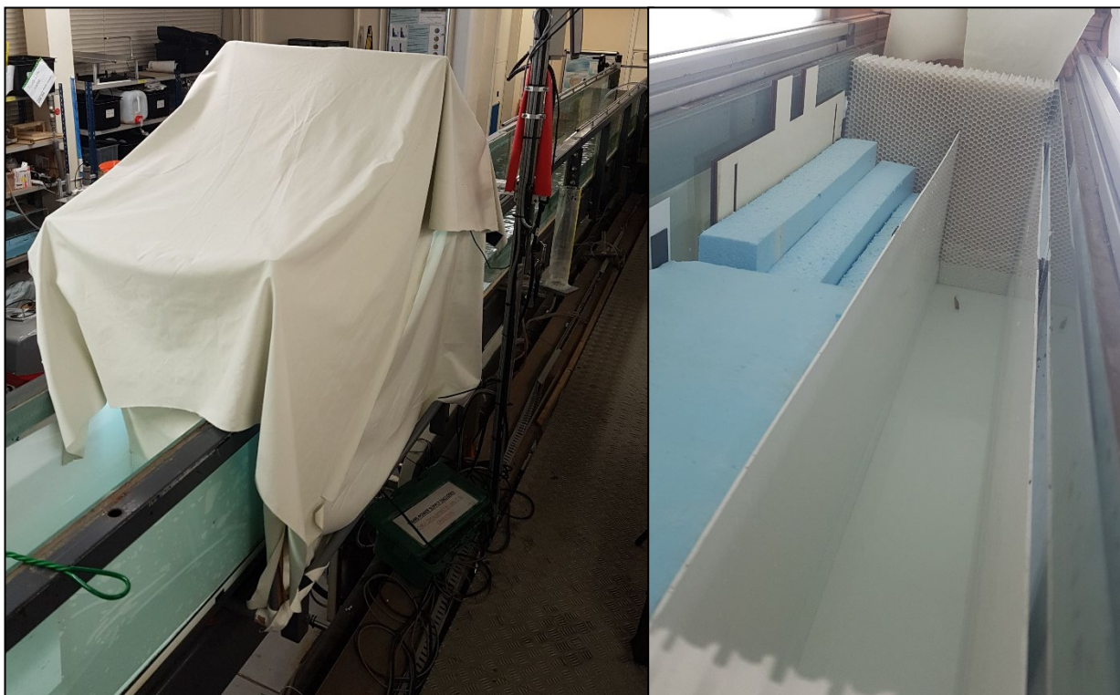
Figure 3.2. Photograph of the experimental set-up in the 12m open-channel recirculating plint flume used for experiments in Chapter 5 and Chapter 7. Experimental flume and hide (left). Experimental channel used (within the hide) in Chapter 5 with minnow (right).
