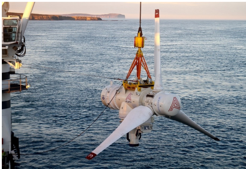
Figure 2.8 AR1500 turbine (Lockheed Martin, 2017)
