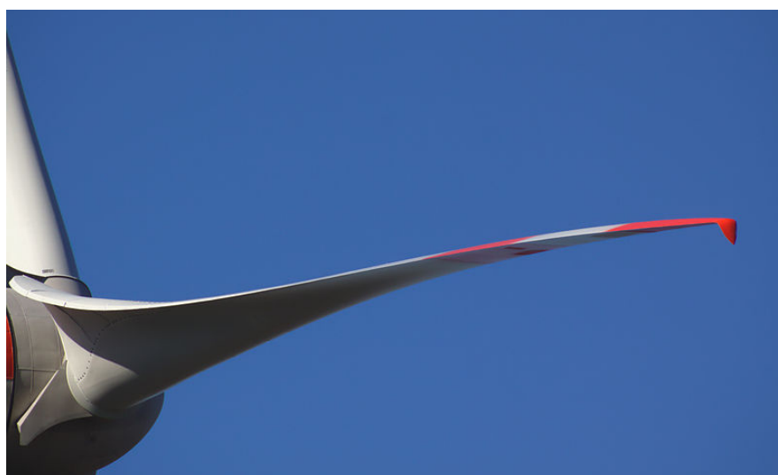
Figure 2.17 ENERCON E-101 turbine with winglets (Aßbrock, 2013).
