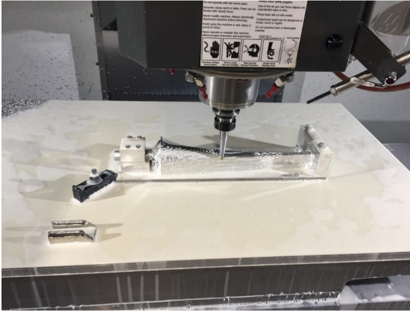
Figure 4.2 CNC machining of a blade from a block of aluminium.
