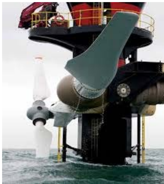
Figure 2.7 Seagen S turbine (SIMEC Atlantis Energy, 2016).
