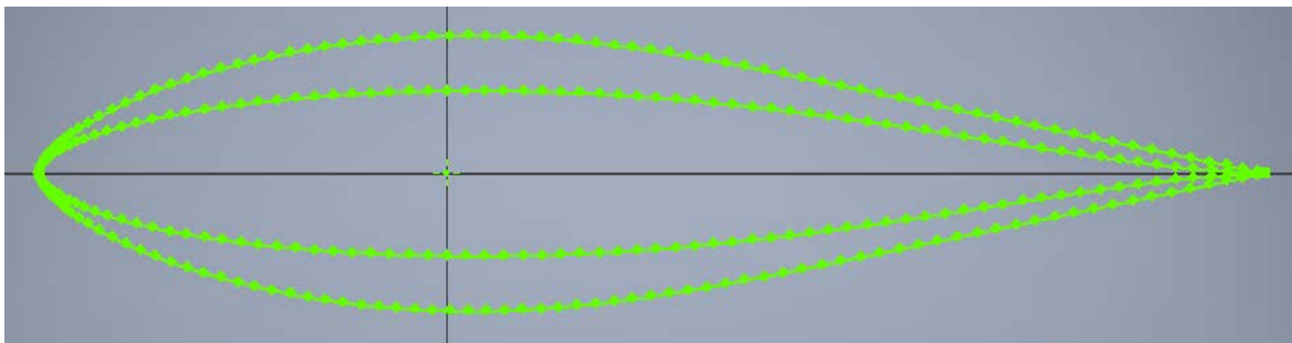
Figure 4.48 Inverted airfoils with aligned centre points (Autodesk screen shot reprinted courtesy of Autodesk, Inc.).
