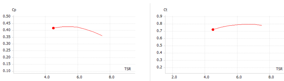
Figure 4.1 Cp and Ct curves from the BEM software simulation.
