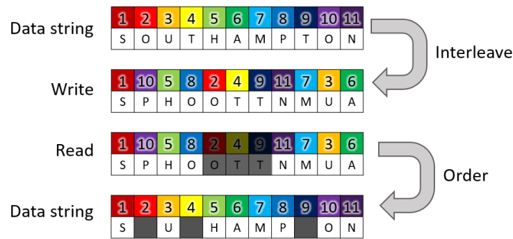
FIGURE 4.9: Visualisation of interleaving to reduce the effect of burst errors: A data string is interleaved, in this case a random order was applied. This string is then written and read out. During read out, a burst error occurred. Since the string is reordered from 1 to 10, the burst error in the middle of the string during read out is now distributed along the whole word.
