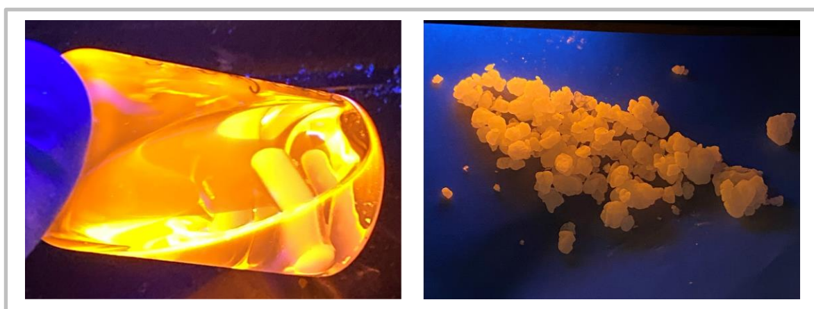
Figure 5.1 Photographs of molten (left) and solid (right) samples of a \text{PbBr}_2 -TOPO complex
