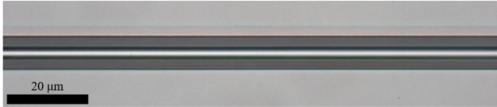
FIGURE 5.6: Microscope image of a well-crystallised polysilicon waveguide, with a smooth and consistent surface along the full length. Losses in this waveguide were measured as 4 \text{ dB cm}^{-1} .
