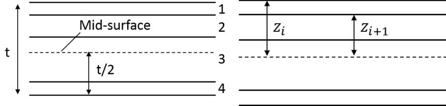
Figure 1: Example of 4-layered laminate panel. Definition of mid-surface and convention of layer's boundary coordinate.
