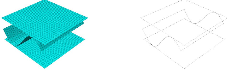
Figure 3: RVE and its external nodes used in Energy-equivalence homogenisation technique
