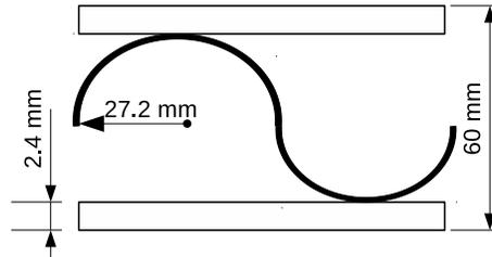
Figure 4: Geometry of analysed sandwich panel
