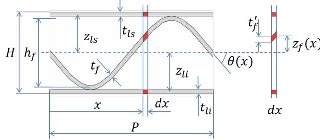
Figure 2: Cardboard section with characteristic CLPT properties annotated.
