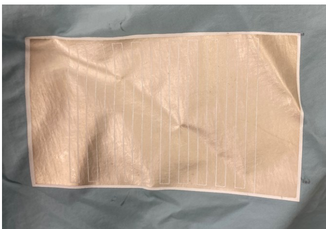
Figure C.5 Photograph of Ag IDEs heat-pressed directly on a garment.
