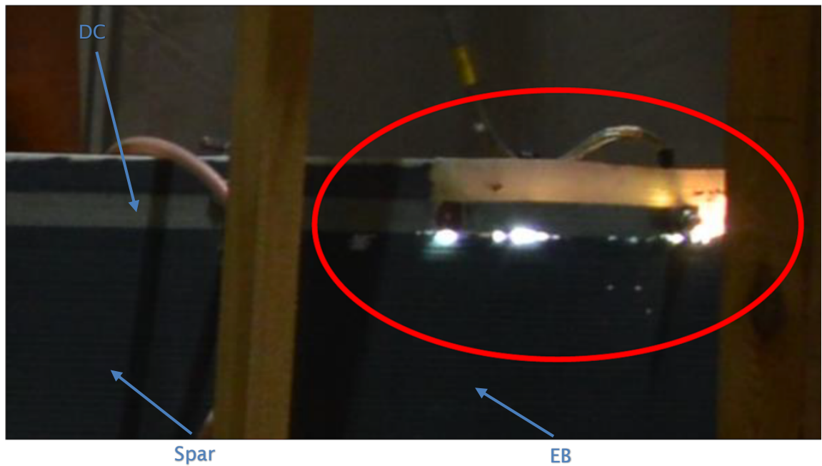
Figure 1.4 – Sparks (circled in red) occurring at the EB region.
