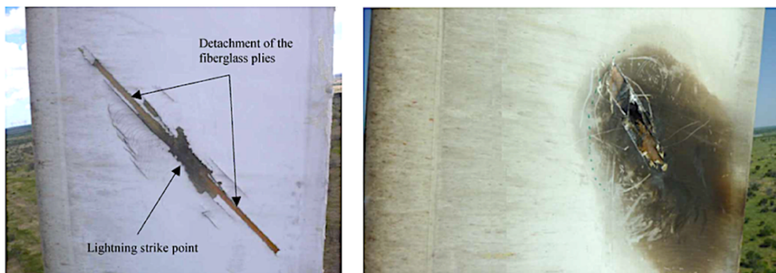
Figure 2.7 – Delamination of the shell plies [22].
