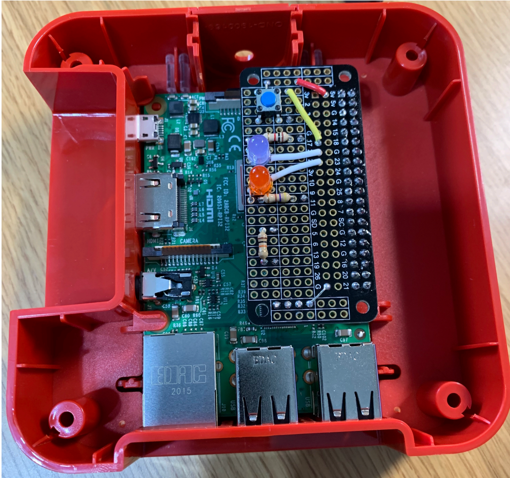
FIGURE 11.2: The experimental hardware, consisting of a Raspberry Pi 3B+ single-board computer, and a custom circuit board.
