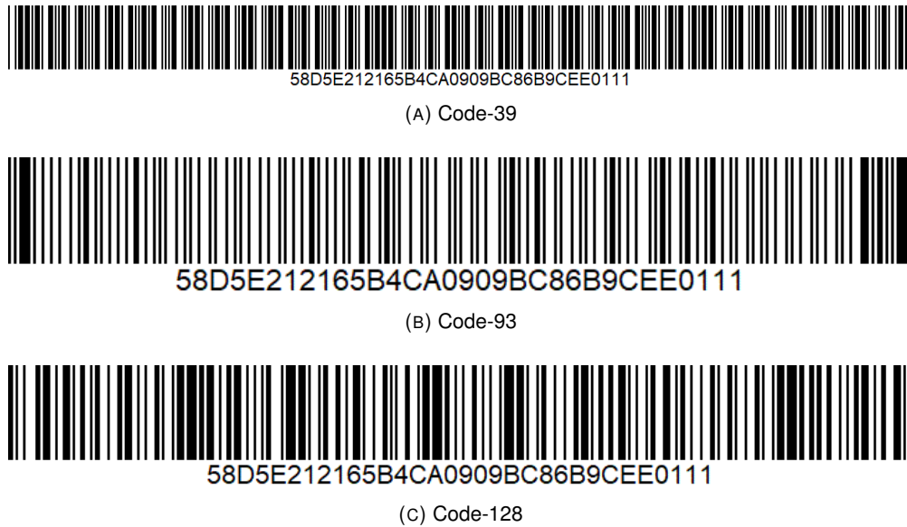
FIGURE 7.13: A 32-character hexadecimal value, rendered in a number of one-dimensional bar code types.
