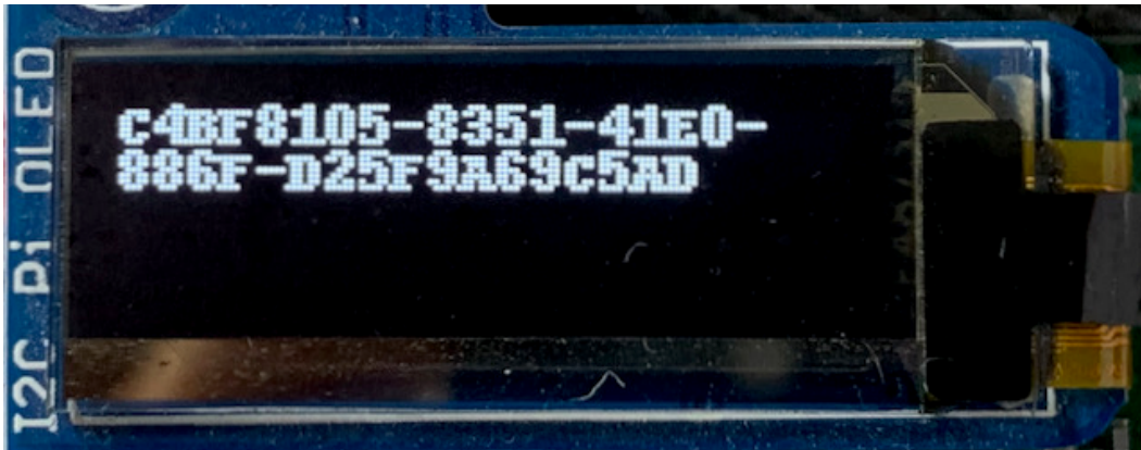
FIGURE 7.5: The 128-bit UUID value, rendered on an OLED screen.
