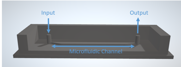
Figure 3.13: 3D model of the microfluidics model, designed with Solidworks.
