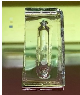
Figure 3.15: An optical microscope image of the PDMS cell bonded onto an SOI chip.
