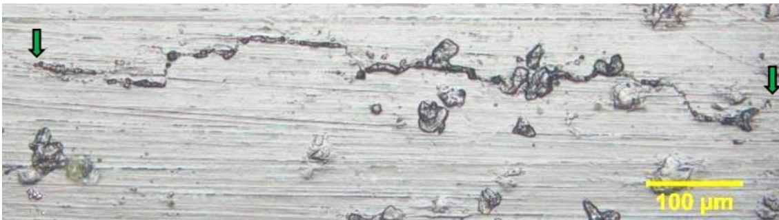
Figure 4-8 A short crack approximately 800 \mu\text{m} in length. The two green arrows show the approximate crack tip locations upon which the crack length is estimated.
