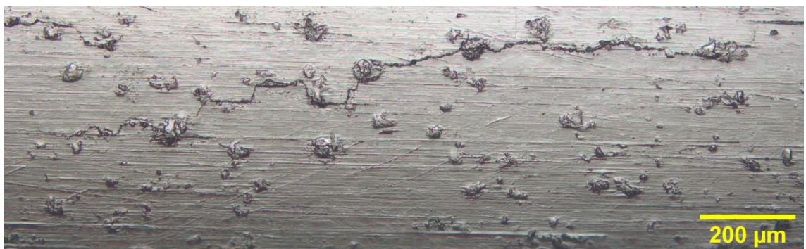
Figure 4-33 Surface replica of as-received surface condition at 74 % lifetime. The central crack can be seen growing through corrosion pits, following machining marks and coalescing with cracks almost parallel with the tensile axis. Crack growth behaviour is less dictated by microstructure and more by surface features than a polished surface condition where these features were removed.
