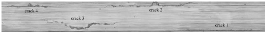
Figure 2-15 Schematic showing the ‘out-of-plane’ distance between neighbouring cracks \Delta Y_k and the crack tip distance between neighbouring cracks from [70]. B) Example of short crack growing ‘out-of-plane’ in a U-notched FV448 material with radius of 2.25 mm [72].
