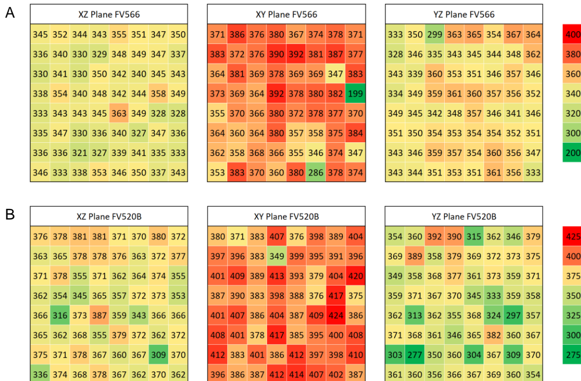
Figure 3-11: Microhardness results in Vickers hardness (HV) on three perpendicular planes of A) FV566 and B) FV520B shown as colour maps. One plane was found to be particularly hard in both materials possibly indicative of rolling direction.
