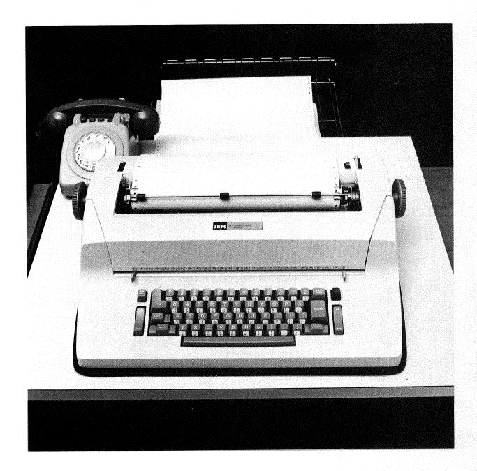
This typewriter terminal is designed for use wherever information has to be passed between a remote location and a central computer (whether the distance is measured in yards or miles). Information entered on the keyboard is transmitted to the computer, and received information is printed out.
