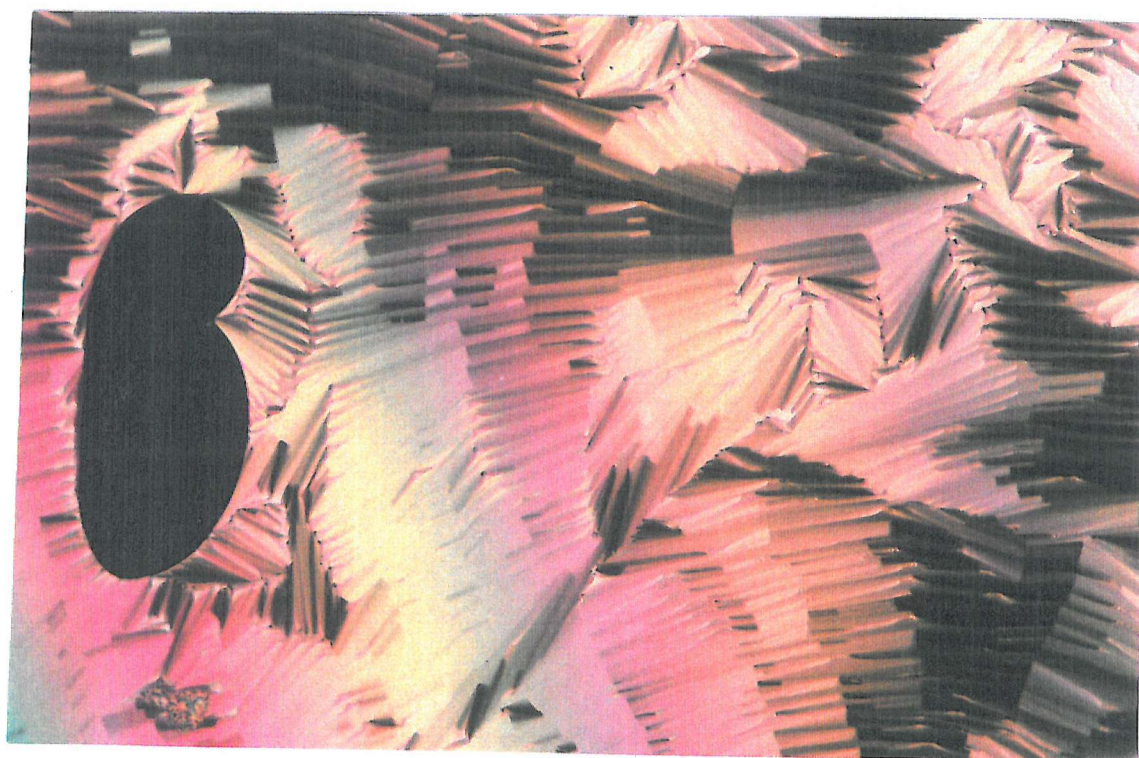
Plate 2. The focal conic fan texture of the monotropic smectic A phase of trimer 6,9 at 128°C. Magnification x100.
