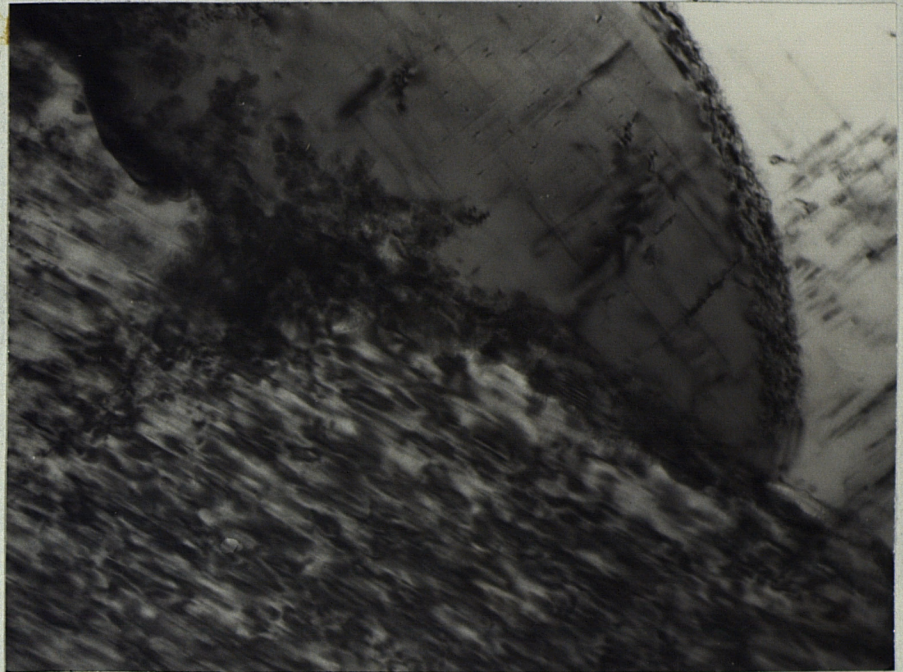
PLATE 7 1000 CYCLE PRESTRAIN BETWEEN S.T. AND AGEING. NON-FATIGUE. (ELECTRON MICROGRAPH x 70K)
