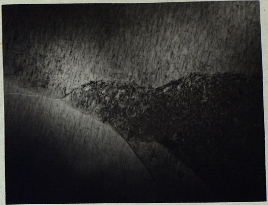
PLATE 9 1000 CYCLE PRESTRAIN BETWEEN S.T. AND AGEING.NON-FATIGUE.(ELECTRON MICROGRAPH x 70K)
