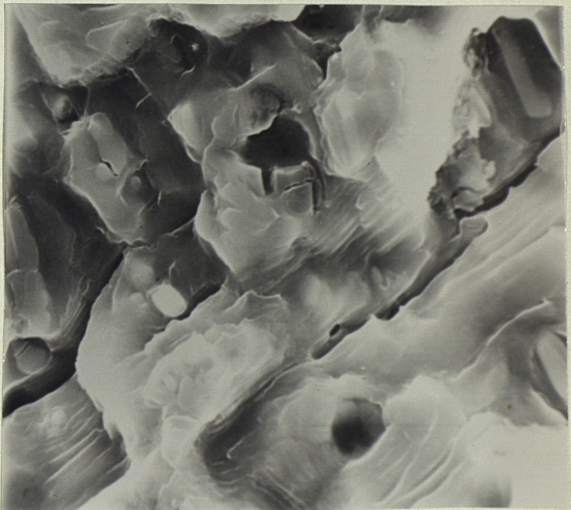
PLATE 20 1000 CYCLE PRESTRAIN BETWEEN S.T. AND AGEING. FATIGUED. (STEREOSCAN x 2.2K)
