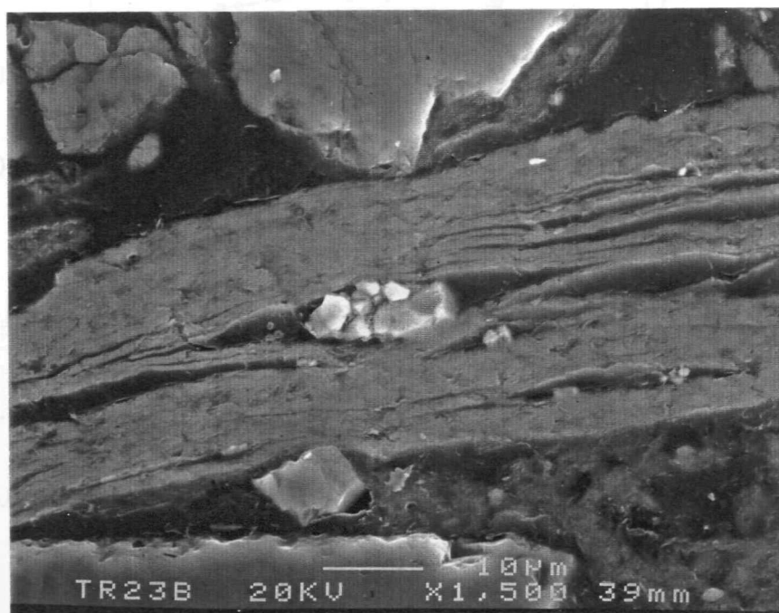
Plate 6-6 SEM image of an Fe/S containing particle within a fibrous elongate clast.
