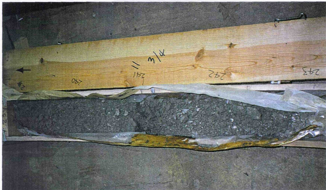
Plate 6-2 Nanjemoy Formation showing poor condition of the core in some intervals.
