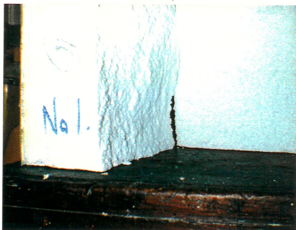
Fig 4.3 Bond failure of the polystyrene core for the first specimen (Tensile test).
