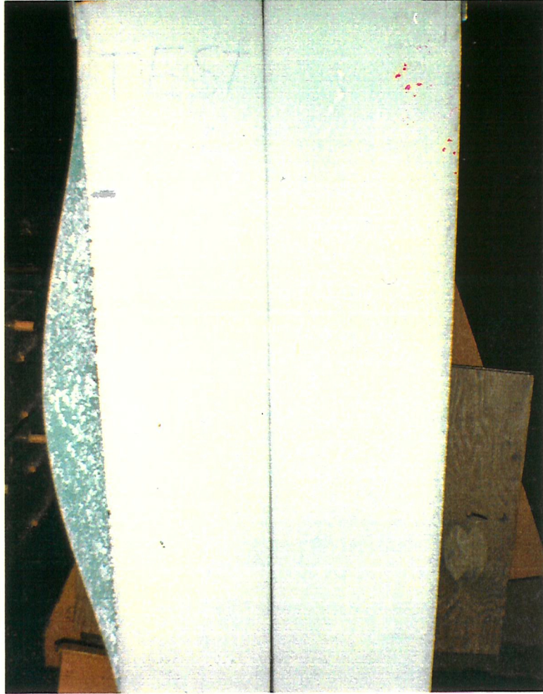
Fig 4.17 Typical bond failure between outer steel faces and polystyrene core (Second shear test)
