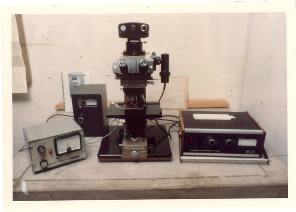
Figure 2.1: Vickers M41 Photoplan Microscope With Light Source, Phototimer And "Microtec" Warm Stage.
