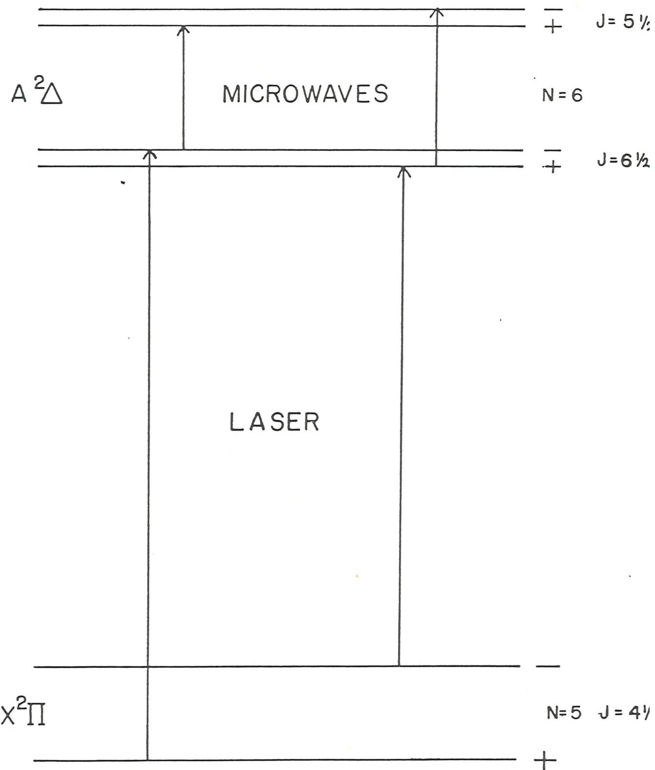
Figure 13. Energy level diagram for the  $A^2\Delta$  state of CH with the possible spin-rotation transitions drawn in. Each of the  $J$  levels shown has two levels split by lambda doubling, each of these being split again by the proton hyperfine interaction.
