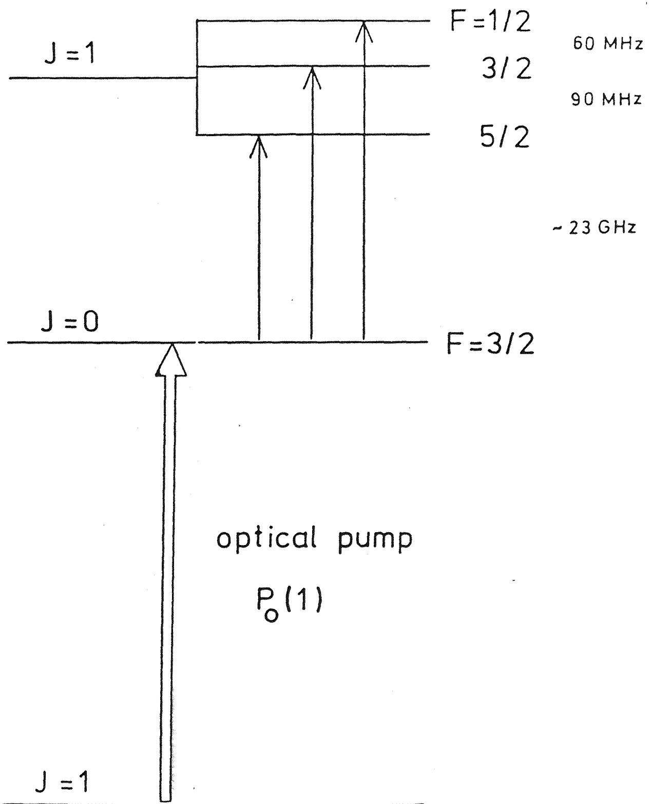
Figure 11. Hyperfine structure on the  $J = 1 - 0$  pure rotational transition in the  $v = 0$  level of CuF  $b^3\Pi_{0+}$ . The three components are due to interactions with the copper nucleus for the  $J = 1$  level. No fluorine hyperfine splitting was observed even at this narrow linewidth of about 5 MHz.
