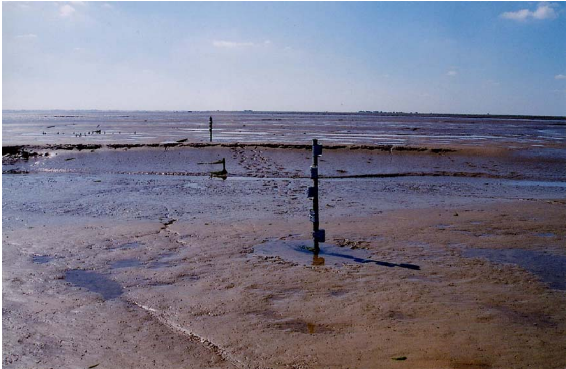
Plate 4.3: A series of (5) suspended sediment samplers attached to a scaffold pole at site 3 during Deployment 4 , at various depths above the bed.
