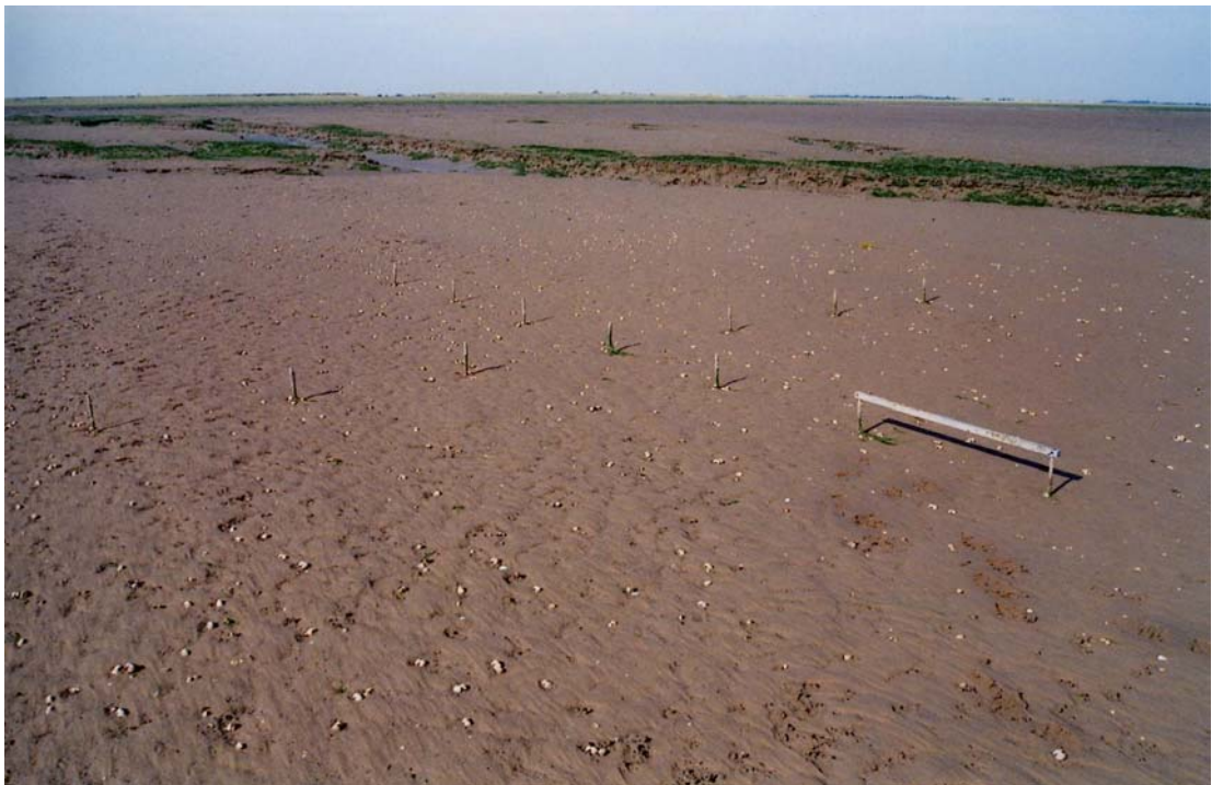
Plate 4.4: The erosion/accretion poles arranged in their 'cross formation' at site 2. The bar used for measuring the levels is in measurement position (Note: the bar is 1 m long).
