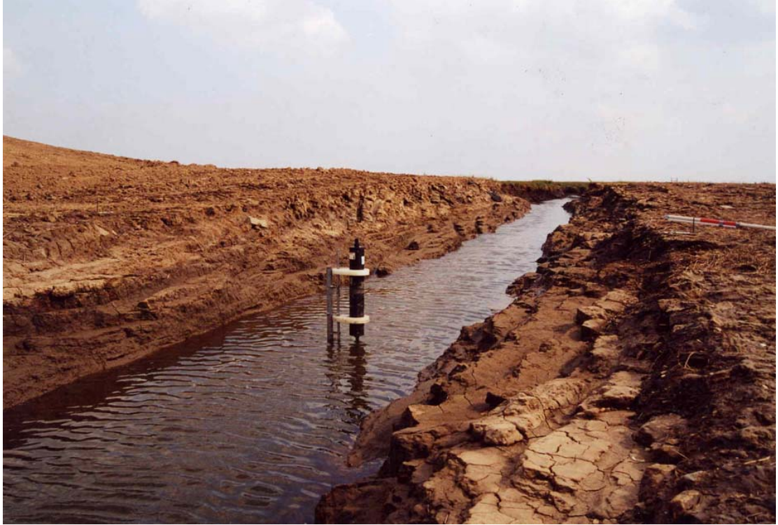
Plate 4.1: The ABR deployed in the channel within Breach 1 (05/09/2002).
