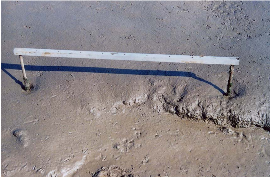
Plate 4.5: The bar used to measure the erosion/accretion rates, positioned between 2 of the poles. Holes in the bar are visible, for the calliper measurements to the bed.
