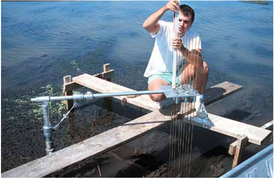
Plate 4.7: Surface elevation measurements of an intertidal mudflat, taken using an SET (from http://www.pwrc.usgs.gov/set/ ).
