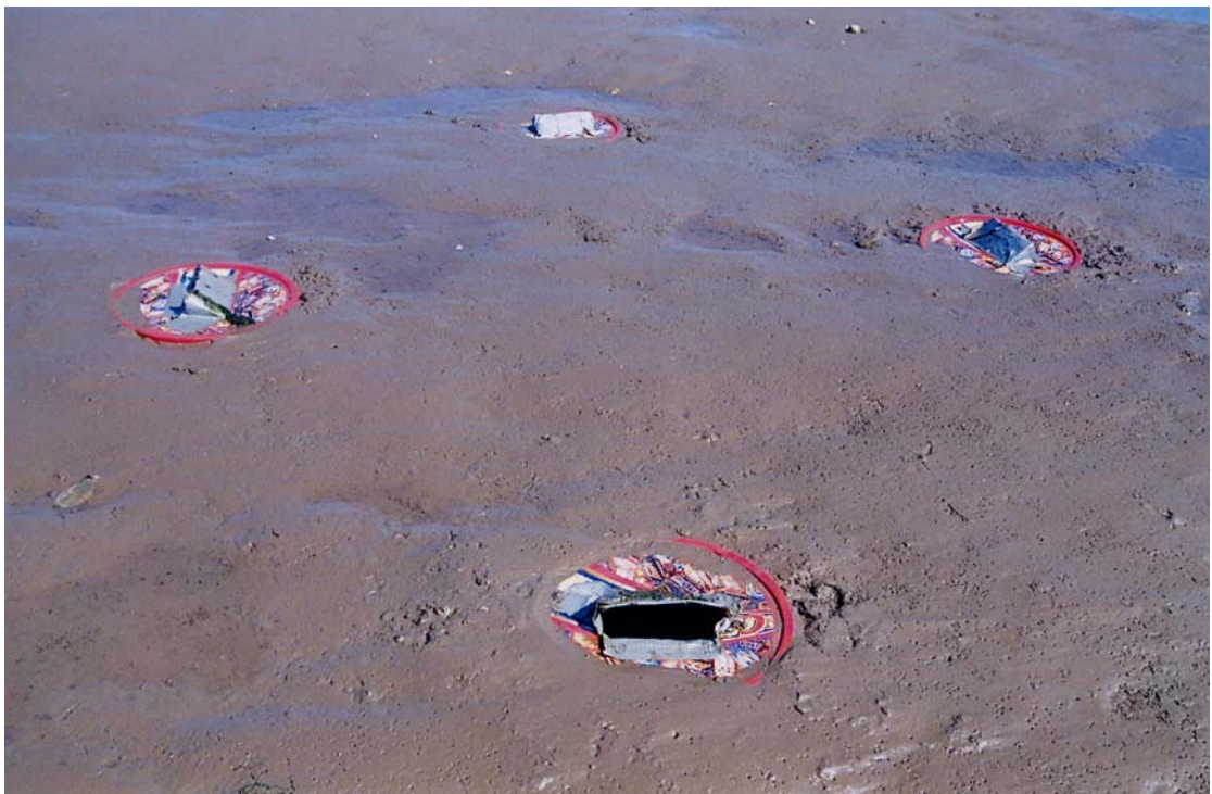
Plate 4.2: A set of 4 bedload traps during Deployment 3 , to collect bedload transport from all directions (Note: the entrance to the trap is 15 cm wide and 5 cm high).
