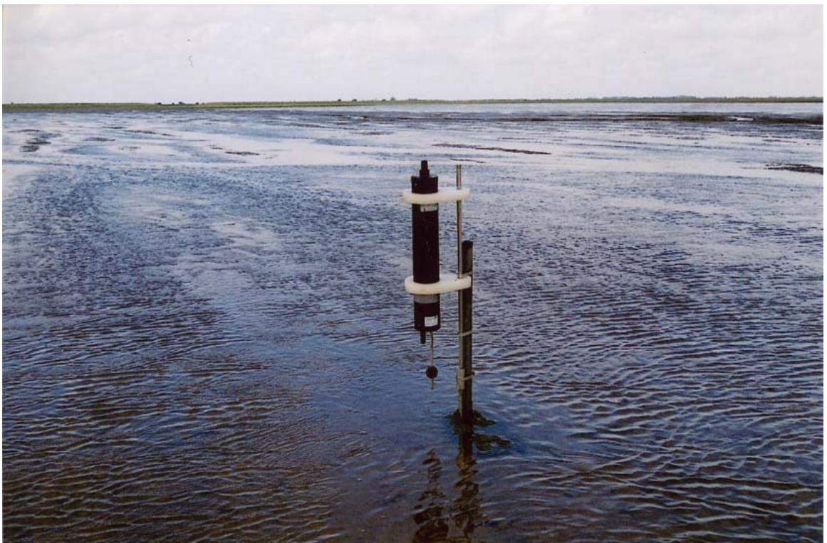
Plate 7.2: The ABR deployed on the lower intertidal site at the start of Deployment 1 (05/09/2002). Note: the whole of the surrounding intertidal flats are flooded, with overland sheetflow.
