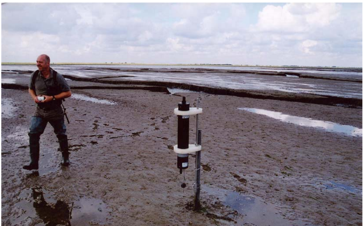
Plate 7.6: The ABR deployed on the lower intertidal site at the end of Deployment 1 (10/09/2002). There is an absence of any overland flow over this area of the intertidal flats, in response to the rapid development of the creek system (visible behind the ABR, in the Plate). Note: compare with Plate 7.2 (see text).
