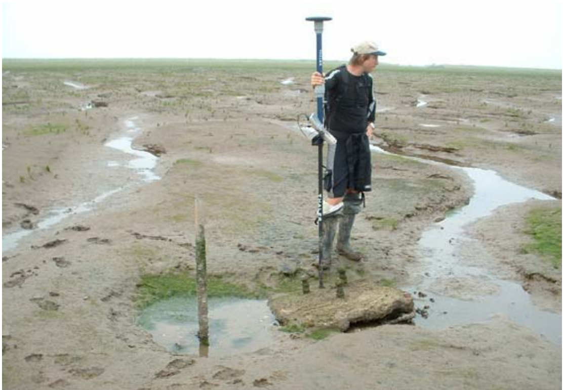
Plate 4.6: The backpack positioning and logging device of the RTK-GPS, recording the location of Base 3, adjacent to the upper intertidal site, site 1 (05/09/2005).
