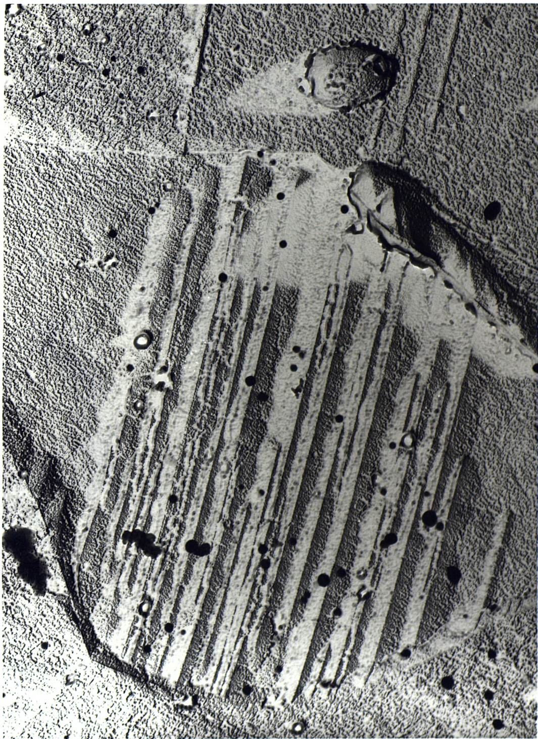
PLATE XXI Surface replica of slip in 18/8 stainless steel fatigue tested at 250°C. x 18000
