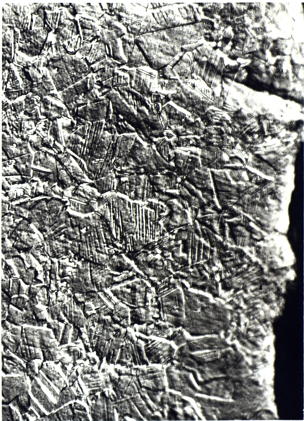
PLATE XX Slip lines in 18/8 stainless steel fatigue tested at 250°C. x 3000
