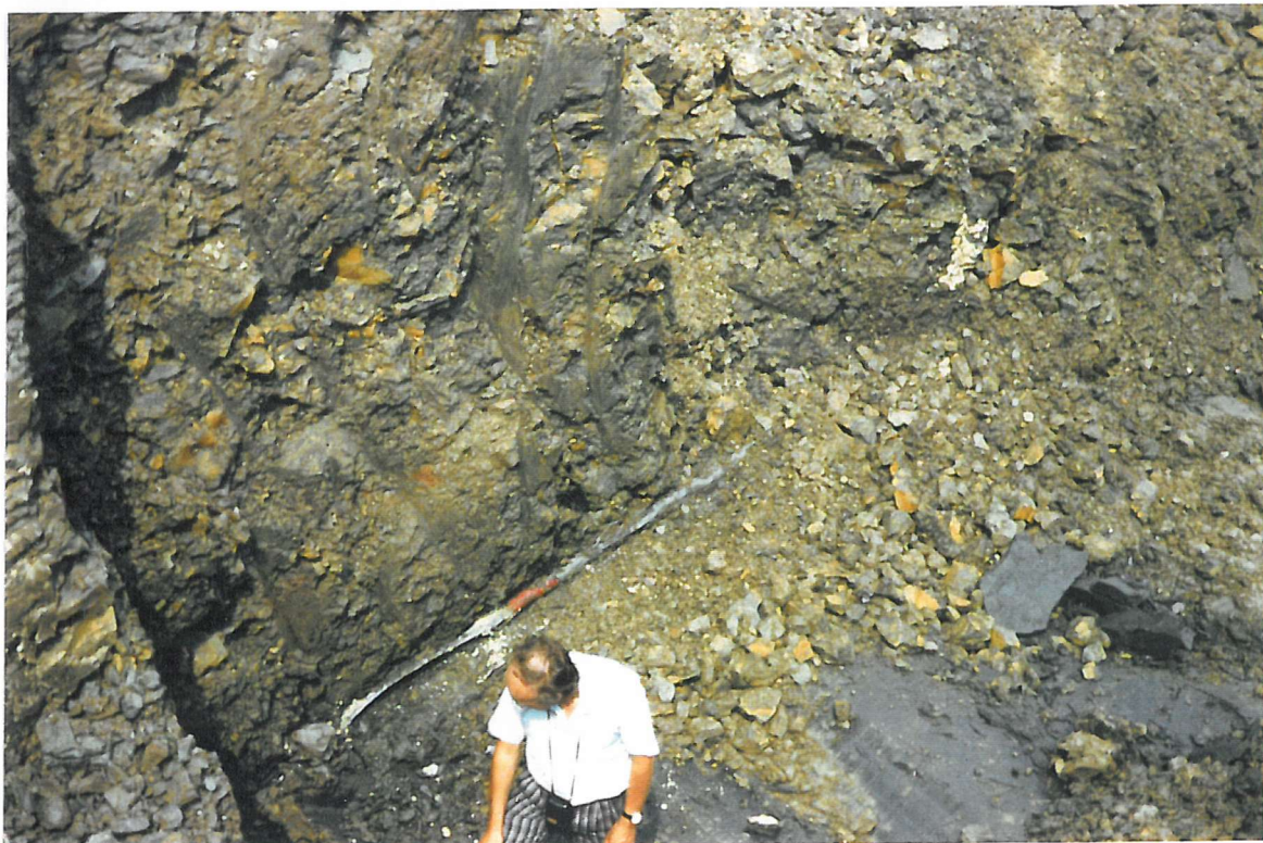
Plate 14-1. Inclinator 07 post failure. Note the access tube laid flat along the slip surface and the empty grout stack still visible towards the upper right of the plate.
