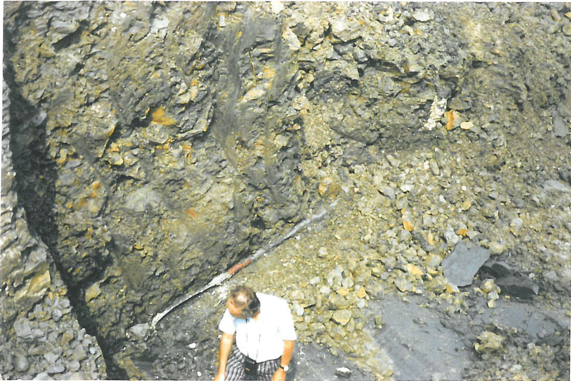
Plate 15-1. Inclinometer 07 laid flat along slip surface.
