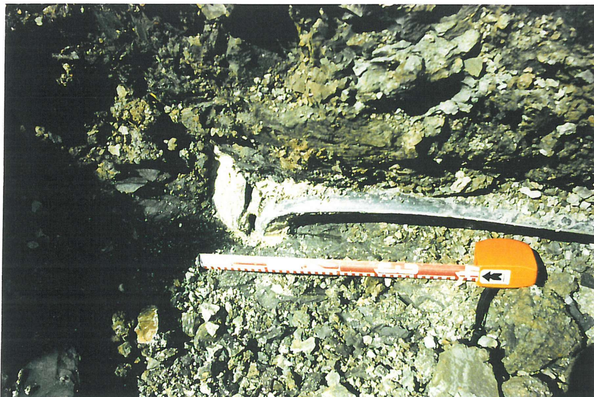
Plate 14-3. Close up of Inclinometer 07 post failure.
