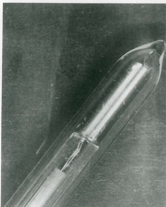
Figure 3-7 Linseis dilatometer specimen holder tube and internal piston.
