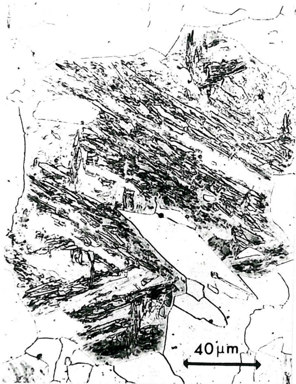
Figure 4-41 E0 quenched out from 650°C
