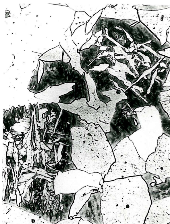
Figure 4-42 E0 quenched out from 600°C
