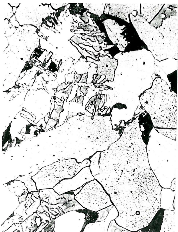
Figure 4-43 E0 quenched out from 550°C
