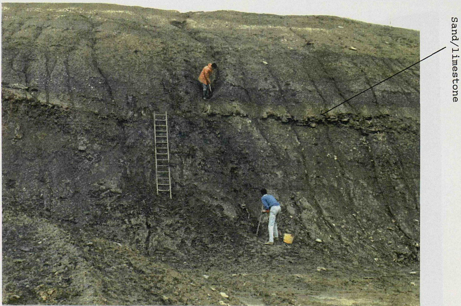
Plate 3.3.1a The northwest sampling section in Langhurst (Warnham) brickwork pits. Sampling work started from the bottom to the top. The sand/limestone bed in the middle is the possible Bed no.11.
