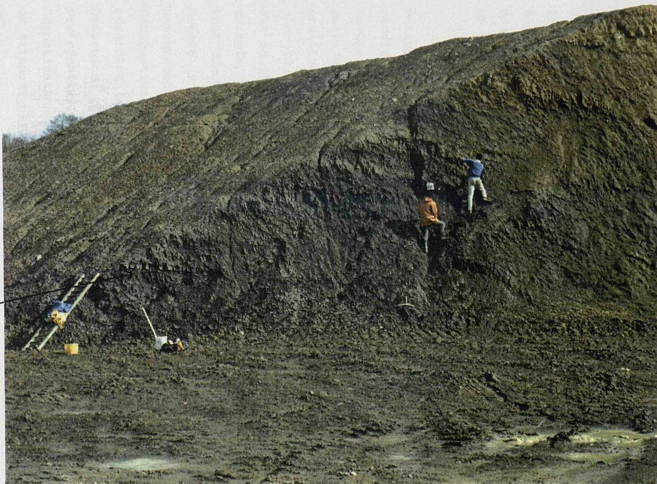
Plate 3.3.1b The southeast sampling section in the same pit. Sampling work was from the bottom to the top. The arrow points the sand/limestone layer near to the bottom, which is the possible Bed no.5.
