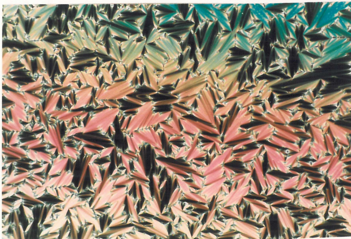
Plate 2.3.4 The paramorphic focal-conic fan texture of the smectic B phase formed on cooling the focal-conic fan texture of the smectic A phase of 4.O4O.4 ( T=140^{\circ}\text{C} ).
