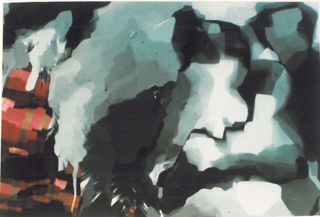
Plate 3.3.3 The arced focal-conic fan and platelet textures of the smectic E phase formed on cooling the smectic B phase of an equimolar mixture of 2OCB and EBBA ( T=48\text{ }^{\circ}\text{C} ).
