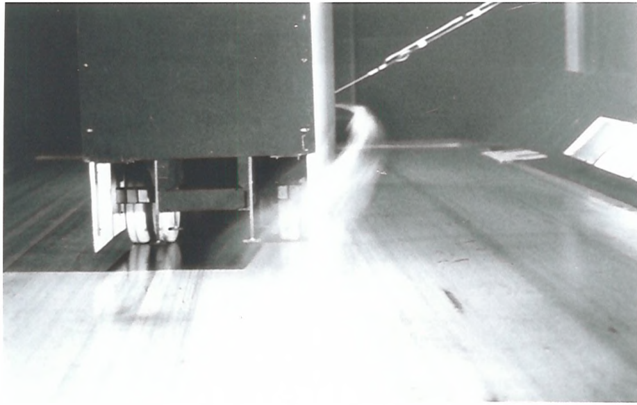
Plate 15(b) 1/4 Scale Fast Front Mk.11 in 3.5m*2.6m Tunnel! Base plus Full Side Skirts 6 Degrees Yaw
