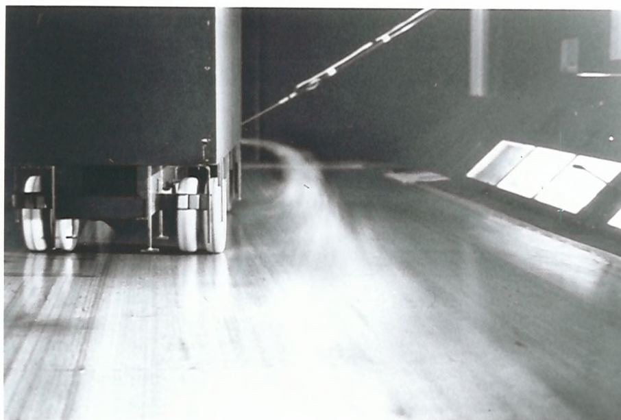
Plate 15(a) 1/4 Scale Fast Front Mk.II in 3.5m*2.6m Tunnel Baseline 6 Degrees Yaw
