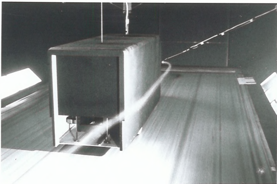
Plate 14(a) 1/4 Scale Fast Front Mk.II in 3.5m*2.6m Tunnel
