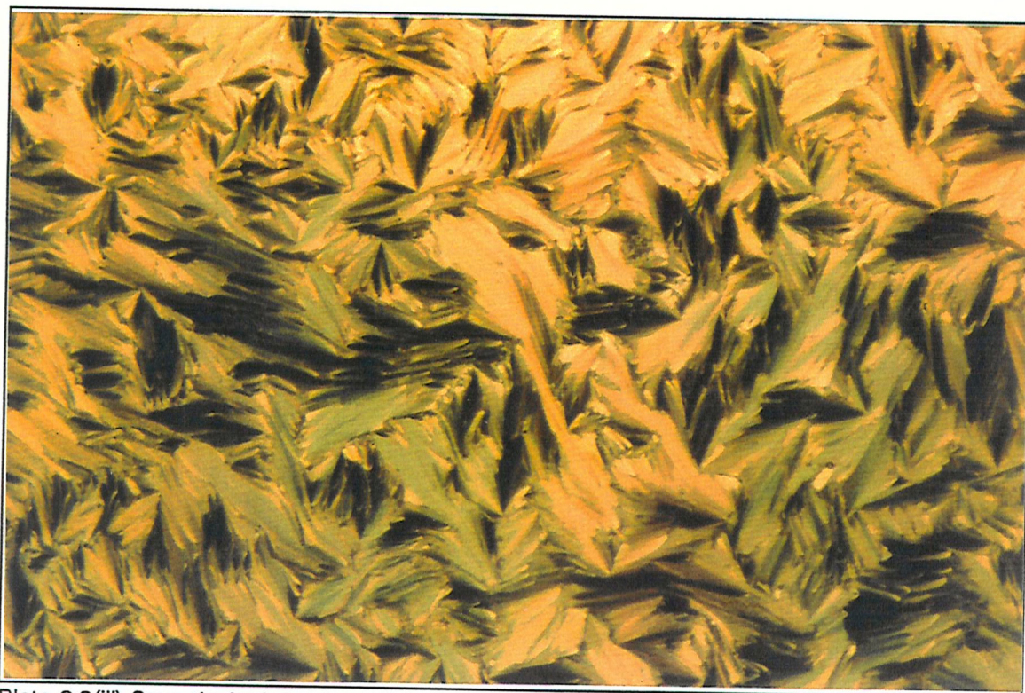
Plate 2.3(iii) Smectic A phase formed by 8-OCT at 213.2°C, showing the focal conic fan texture.
