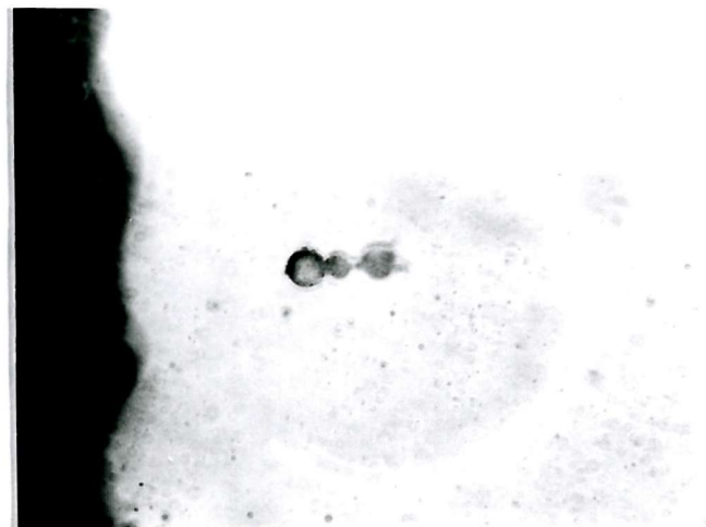
b. Pearl chain bouncing at the negative electrode (magnification x 130).
