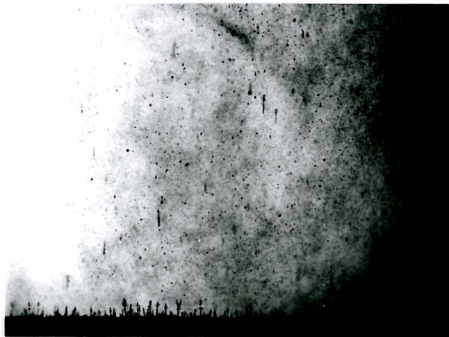
g. Pearl chains and trees attached to the negative electrode (see h.) (magnification x 27).
