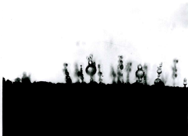
i. Pearl chains and trees attached to the negative electrode - diameter of largest droplet \sim 45\mu\text{m} (magnification \times 130 ).
