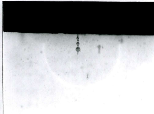
f. A solitary pearl chain attached to the positive electrode - an unusual event (magnification x 130).
