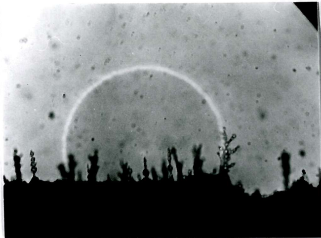
e. Pearl chains and trees attached to the negative electrode (magnification x 130).
