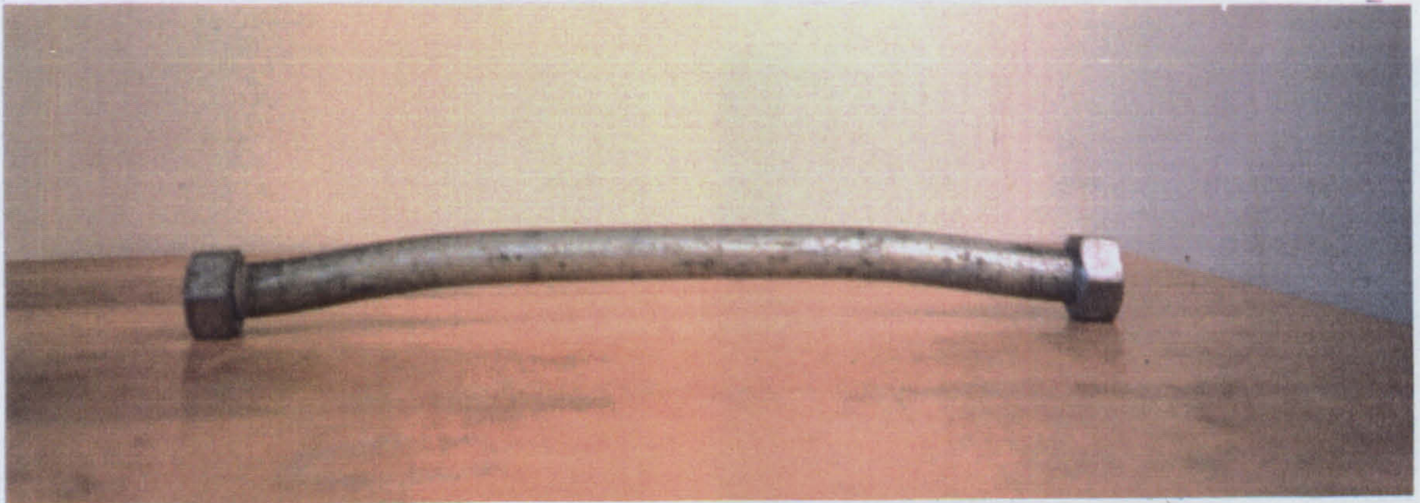
PLATE (3.2) : LARGE DEFORMATIONS EXPERIENCED BY A BOLT AFTER TESTING.
