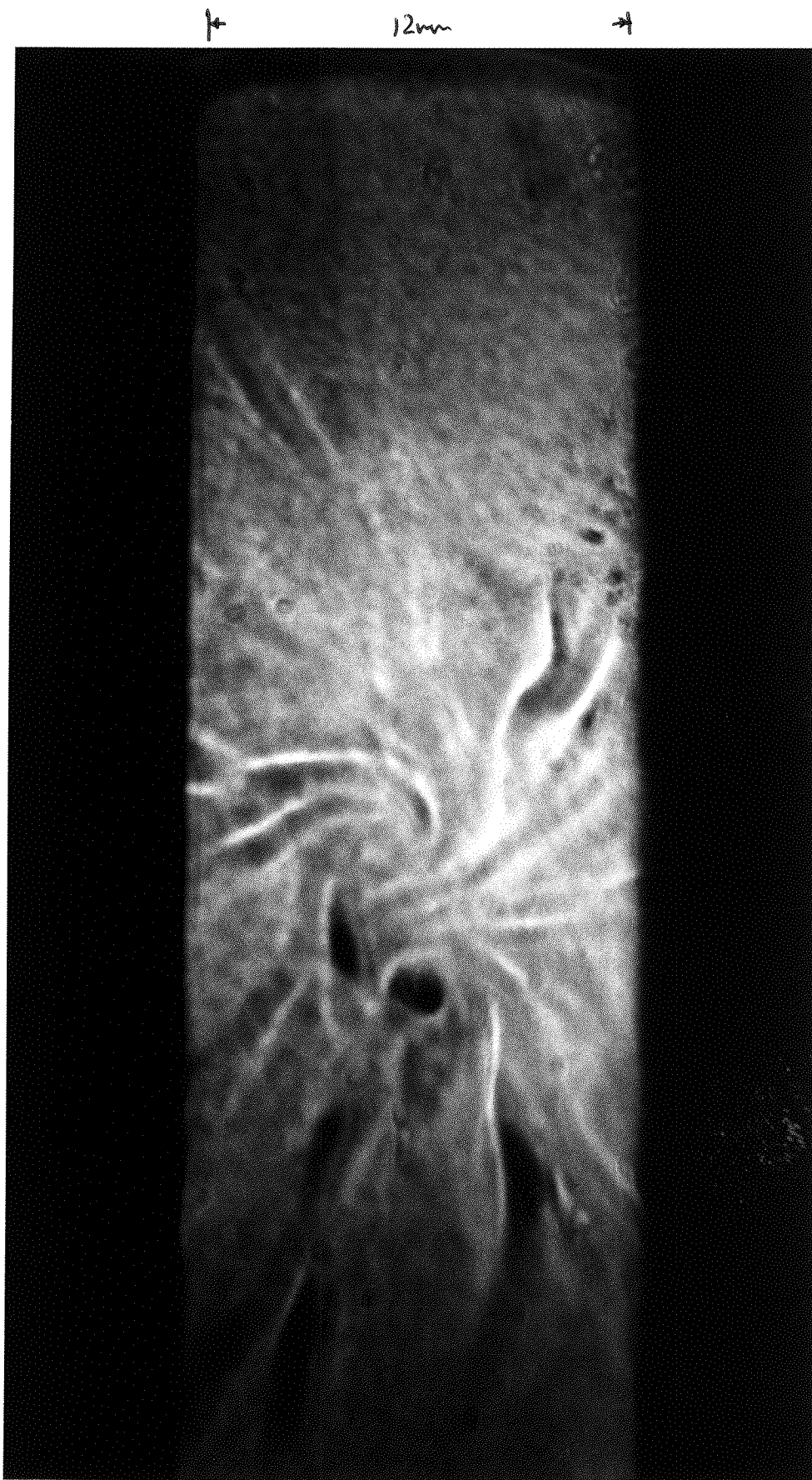
Fig. 31 Schlieren Image of LIN in a 50mm Diameter Vessel with an Evaporation Rate of 200 cc/min. \text{g/s N}_2 at S.T.P
