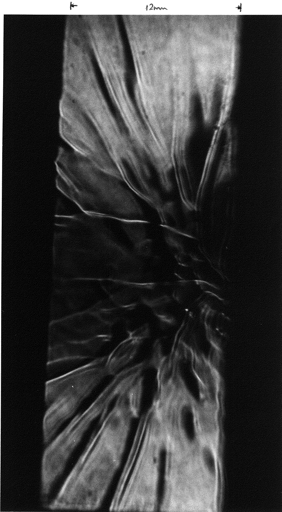
Fig. 34 Schlieren Image of LIN in a 50mm Diameter Vessel with an Evaporation Rate of 900 cc/min. gas N_2 at S.F.P
