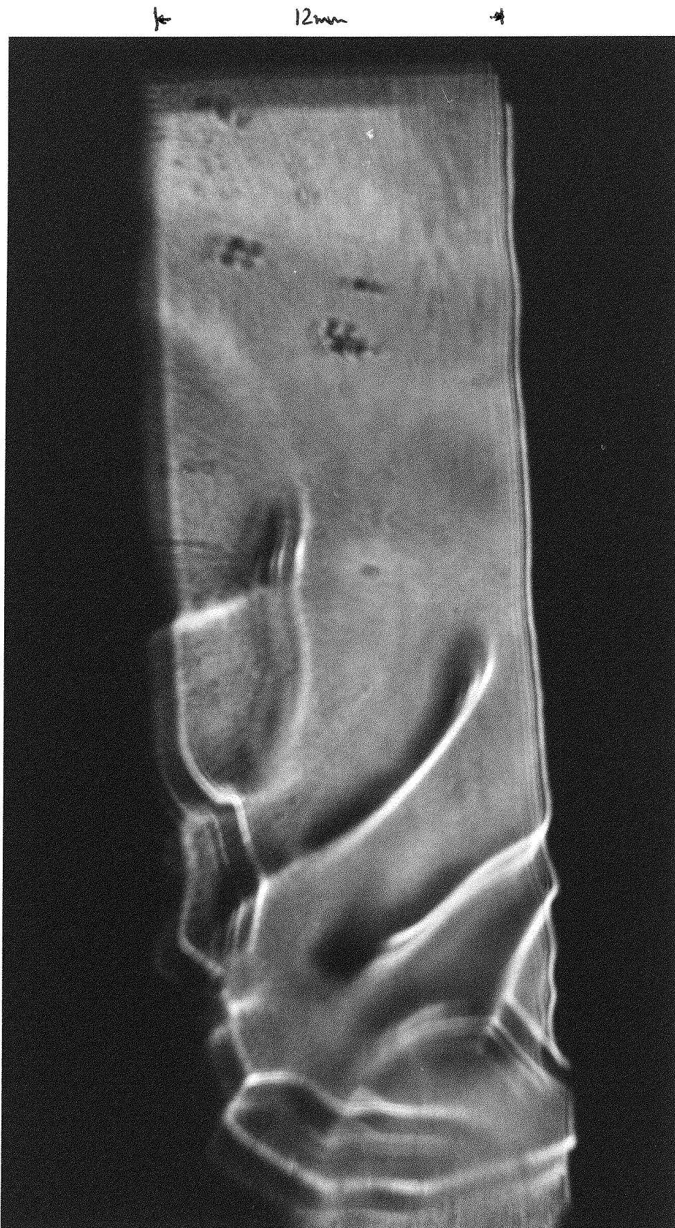
Fig. 32 Schlieren Image of LIN in a 50mm Diameter Vessel with an Evaporation Rate of 400 cc/min. gas N 2 at S.T.P
