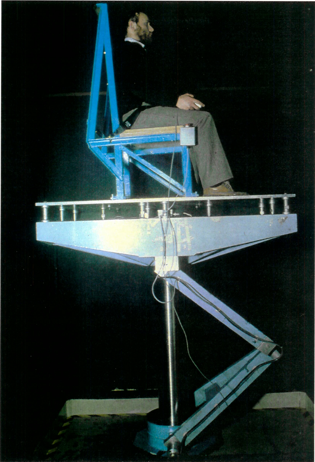
Figure 1.8 The 1 metre stroke vertical vibrator at the University of Southampton
