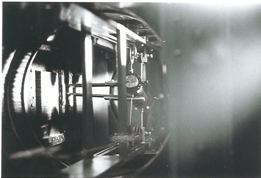
Fig. 3.1 Launching a model during static calibration
