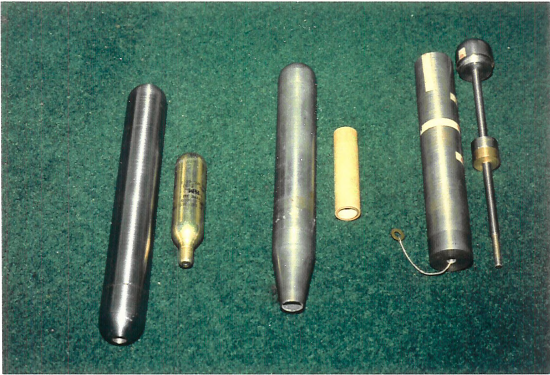
Plate 1: Compressed gas and solid rocket exhaust simulators and representative model
