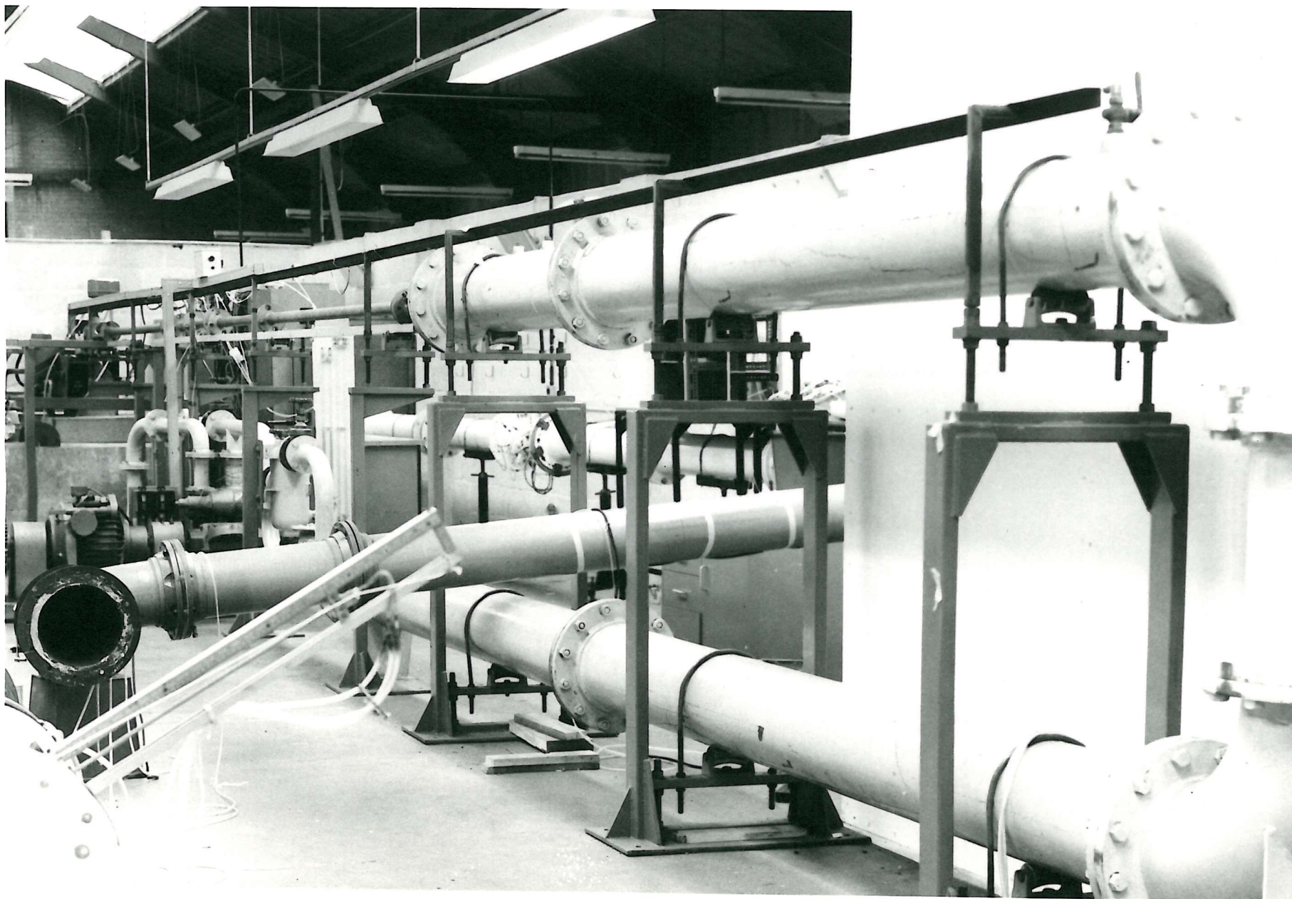
Fig. 2.5 Calibration Rig Showing the 10" dia. Pipe and the 2" dia. Test Length
