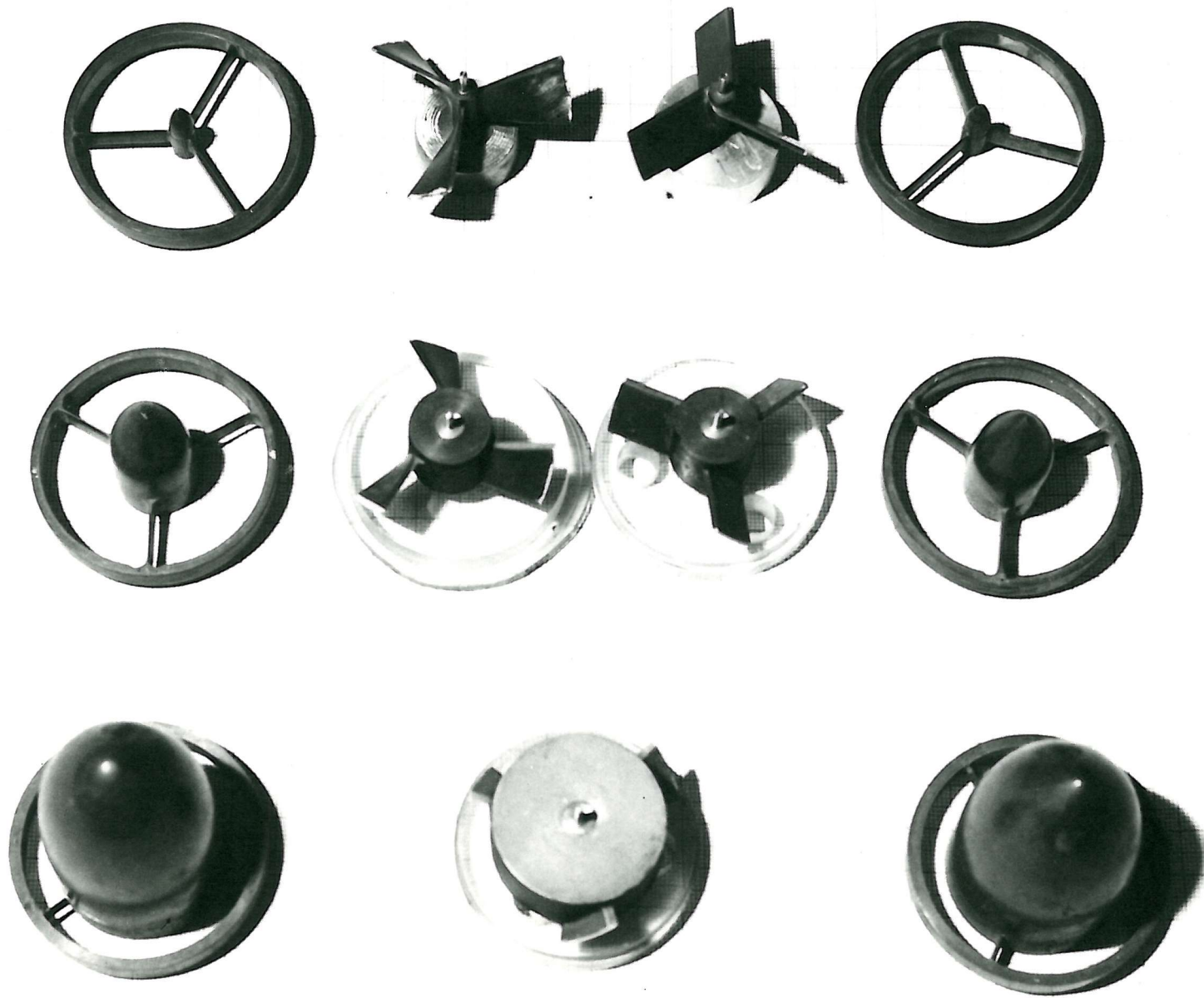
Fig. 5.17 \frac{1}{4} ", \frac{5}{4} " and 1\frac{1}{2} " Hub dia. Research Rotors with Bearing Housings
