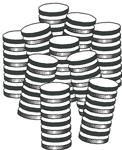
Figure 10. The arrangement of the molecules in a columnar nematic phase. A binary mixture of electron donor (black) and electron acceptor (grey) molecules induces the formation of the columns via charge transfer interactions.
