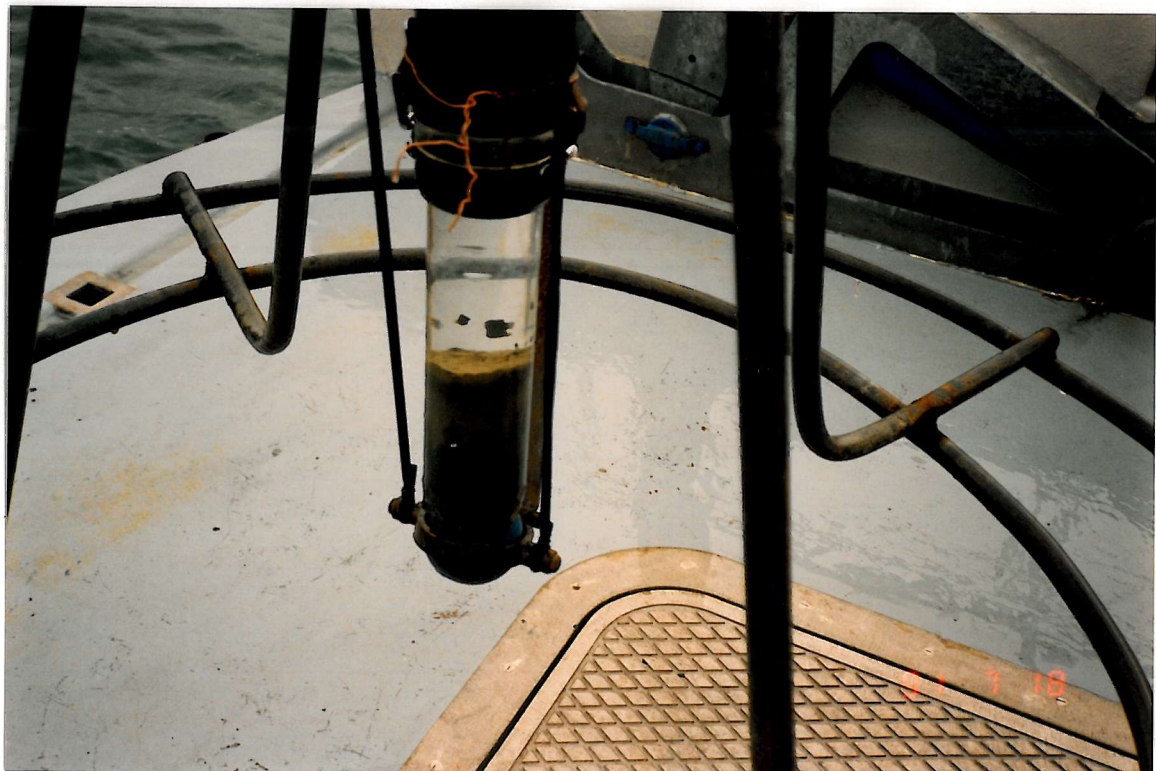
Plate 2 : The sampler being brought up on deck (upper) and the core tube showing a sample collected (some 10 cm in length), with overlying waters (lower).
