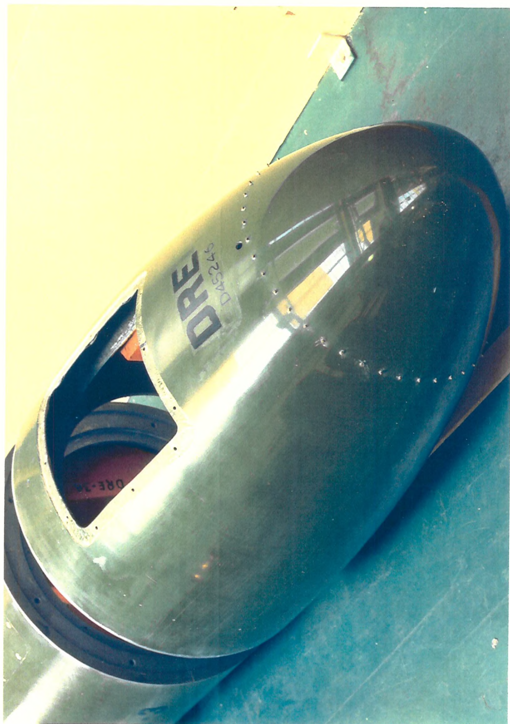
FIG.6 TURBULENCE PINS ON THE NOSE OF A MODEL
