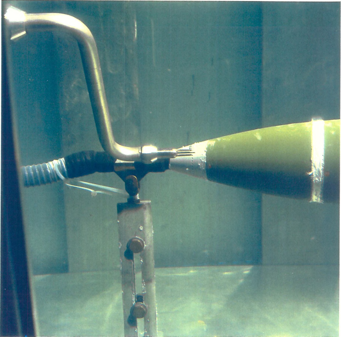
FIG.27 FREESTONE PROBE AT REAR OF MODEL 1990 BLISTERS ARE VISIBLE ON REAR OF MODEL
