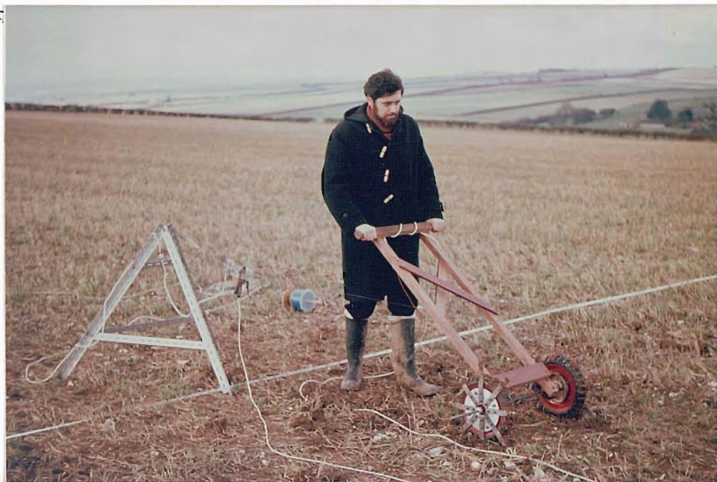
FIG. 7.20. The wheeled resistivity apparatus in use. To the left can be seen one of the tripods of the distance transducer system
