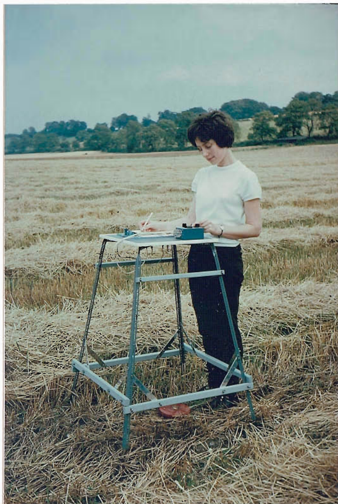
FIG. 4.3. The prototype square array in use before the changeover switch had been added
