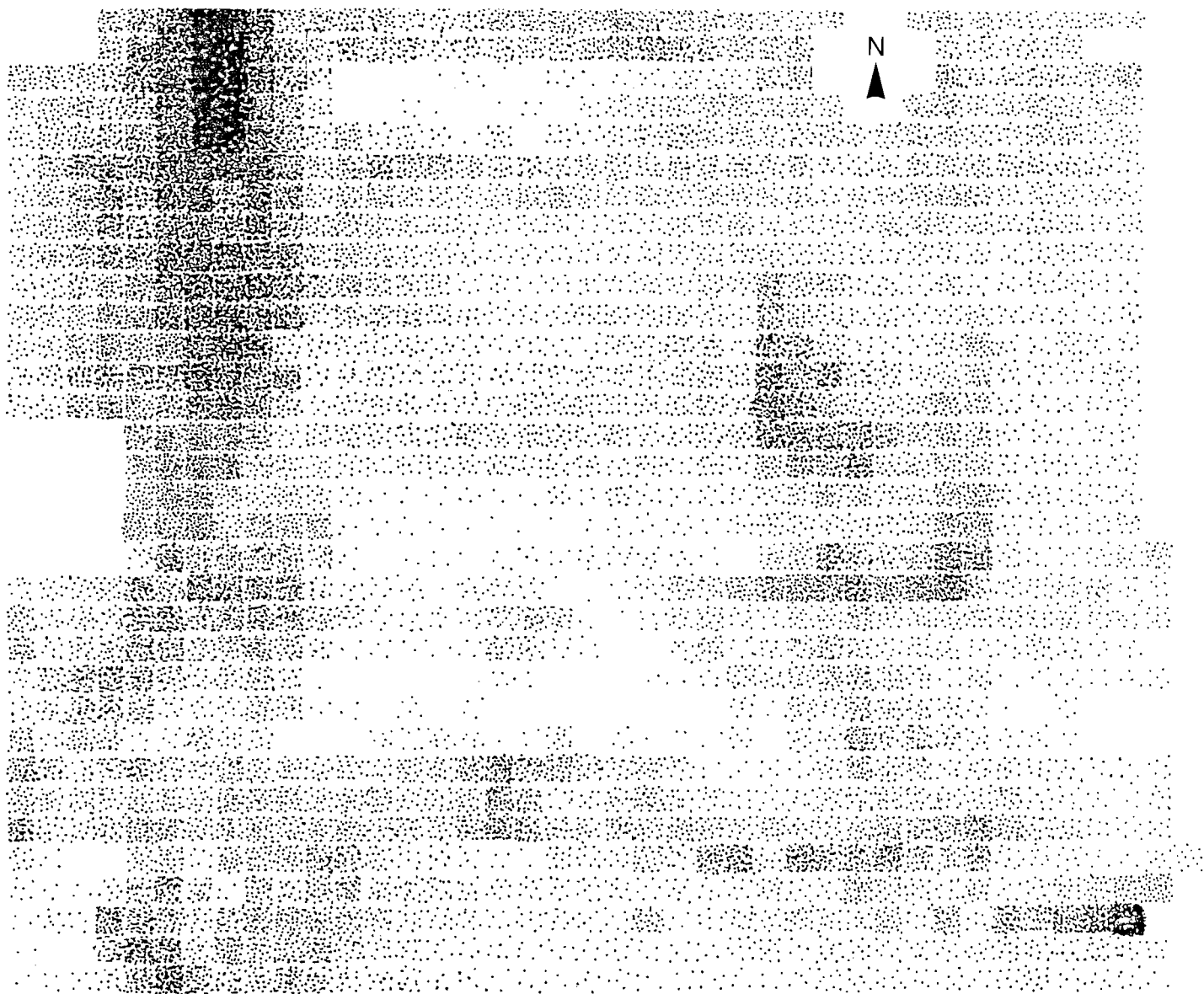
FIG. 7.12. Guildford Park Manor. Manual dot density plot. The plotting cells (i.e. individual readings) are 1 m wide
