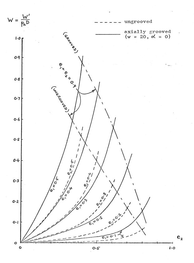
Fig.27 Variation with eccentricity of bearing force per unit length in ungrooved and axially grooved infinite length journal bearings
