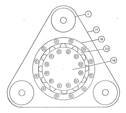
Fig.54 View looking down on the lower bearing plate with the probe tripod and feet removed
