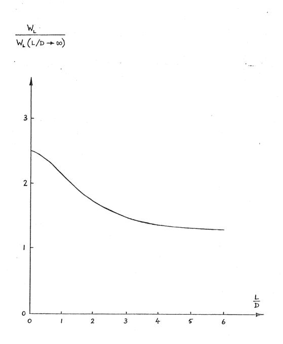
Fig.6 <u>L/D dependence of bearing force per unit length</u> in ungrooved cylindrical bearings
