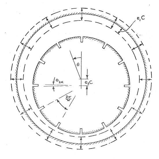
Cross-section of axially grooved journal bearing
