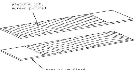
tape of un-fired piezoelectric material
