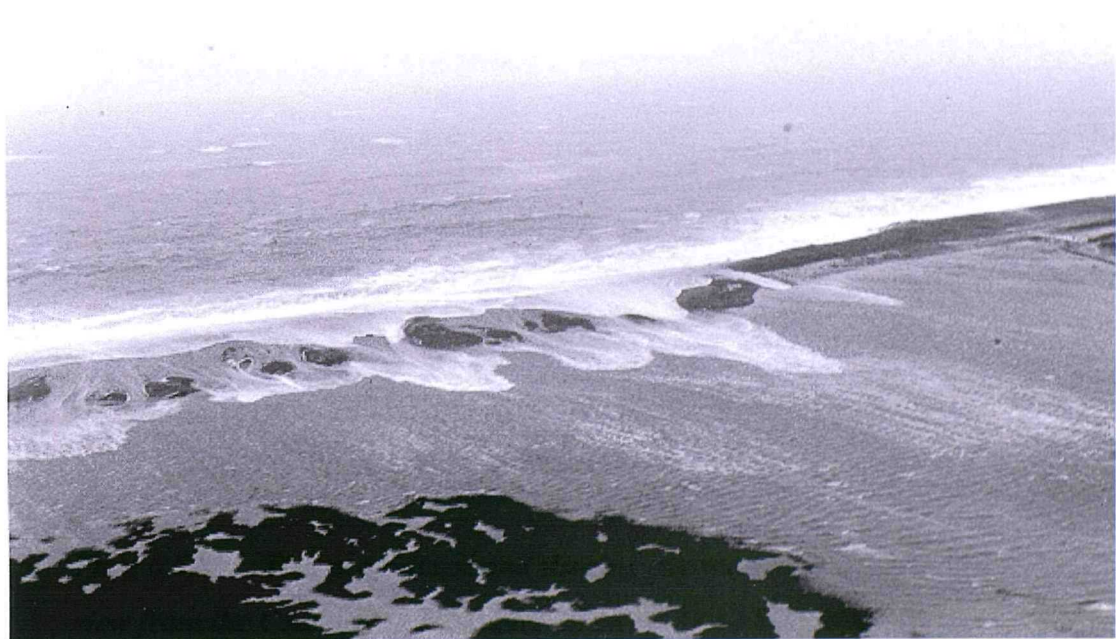
Plate 6.6 Throat confined and sluicing overwashing on Hurst Spit, - aerial view from the Coastguard helicopter taken on 18/12/89 - following the storm peak.
