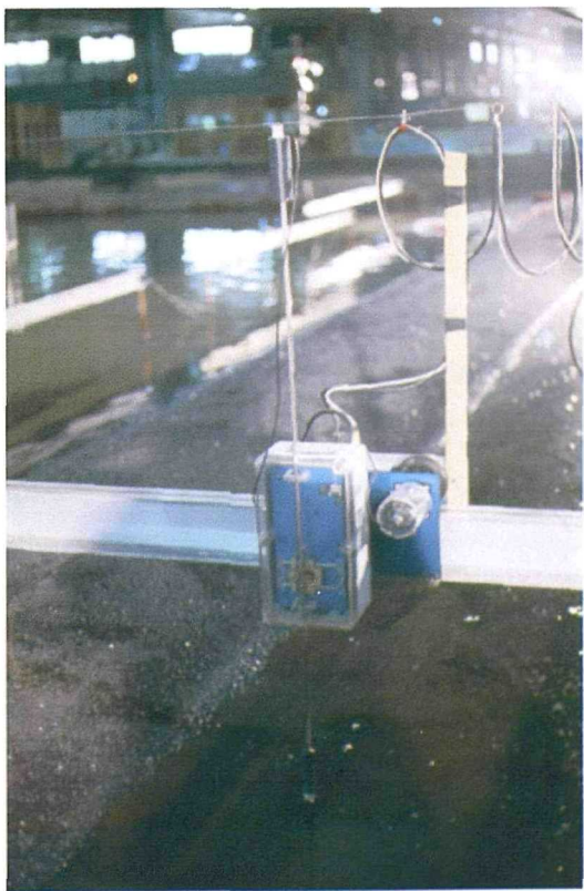
Plate 4.2 Details of the bed profiler used in the model tests, at HR Wallingford
